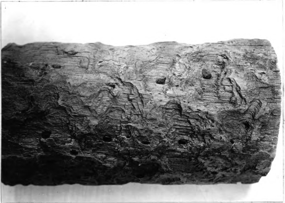
Sawyer work in sapwood of jack pine. Note nearly circular exit holes of adults and the more flattened entry holes of larvae.
