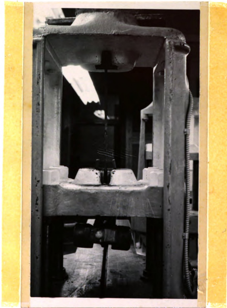
Fig. V Method Used for Clamping Steel Reinforcing Bars in Riehle Universal Testing Machine
