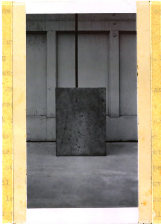
Fig. IV Typical Specimen With Embedded, Hooked, Steel Reinforcing Bar
