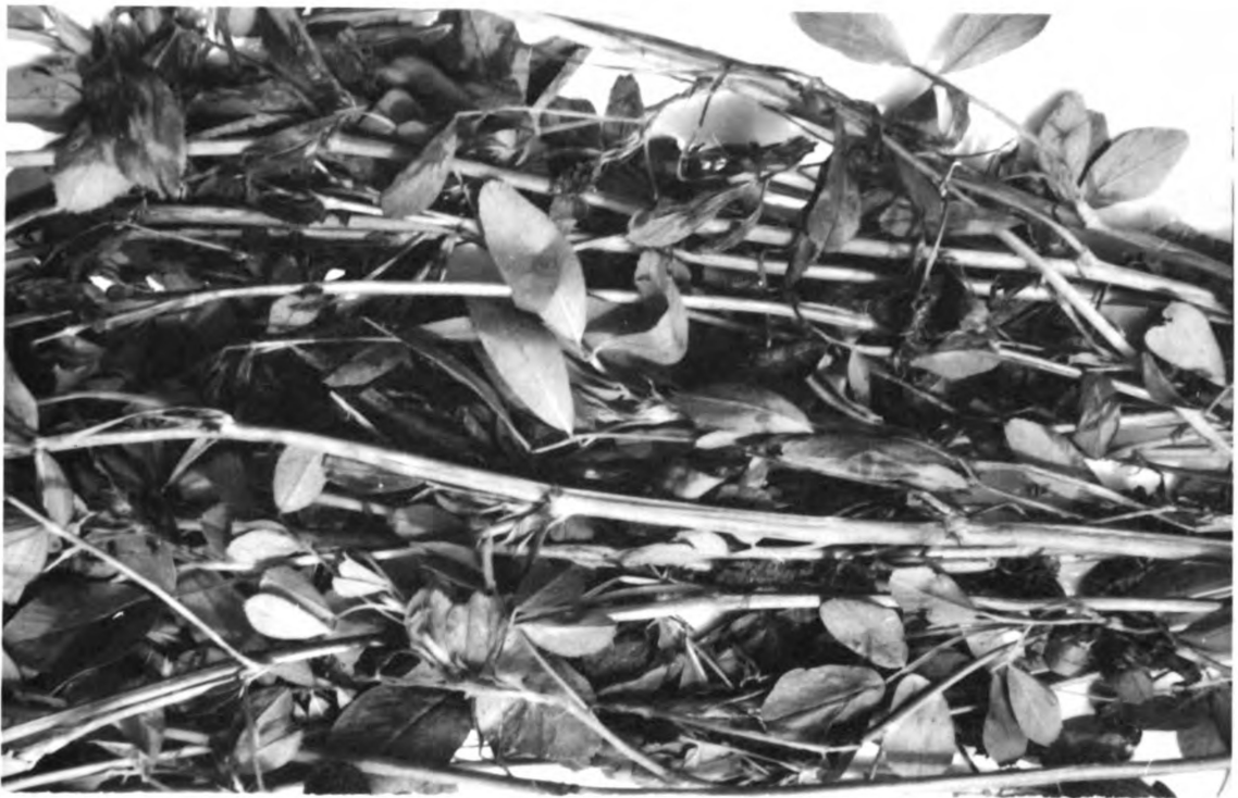
Alfalfa crushed at clearance 0.025 inches.
