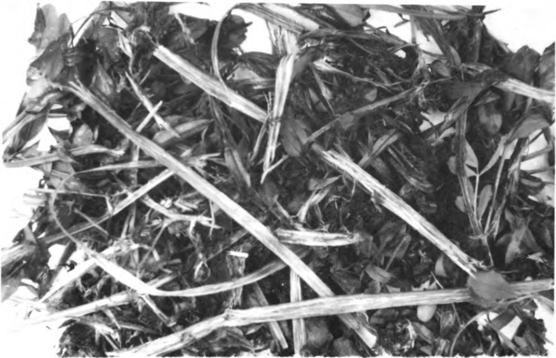
Alfalfa crushed at clearance less than 0.005 inches.
