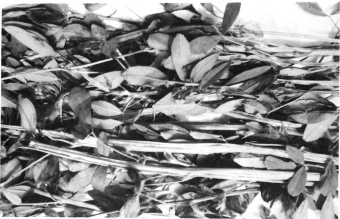
Alfalfa crushed at clearance 0.0125 inches.
