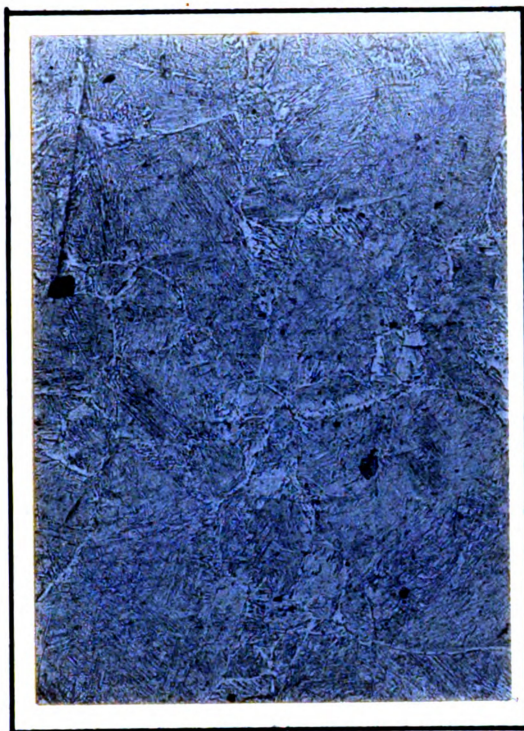
Fig.33. Cooled .12 minutes thru critical temperature.
