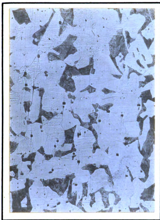
Fig.29. Cooled 33 minutes thru critical temperature.
