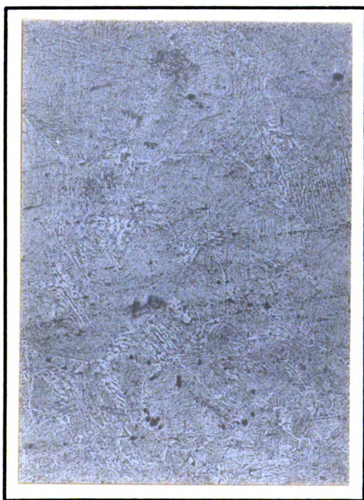
Fig.31. Cooled .4 minute thru critical temperature.
