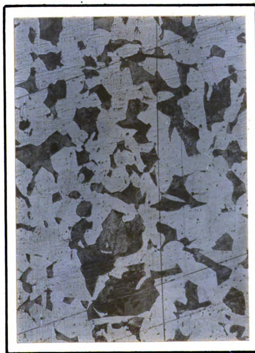
Fig.35. Furnace cooled 1900°F.
