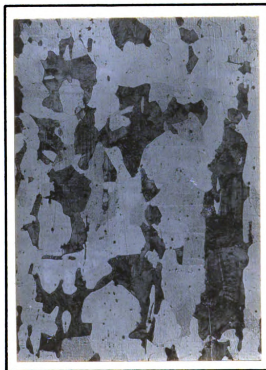
Fig.28. Cooled 2 hours thru critical temperature.
