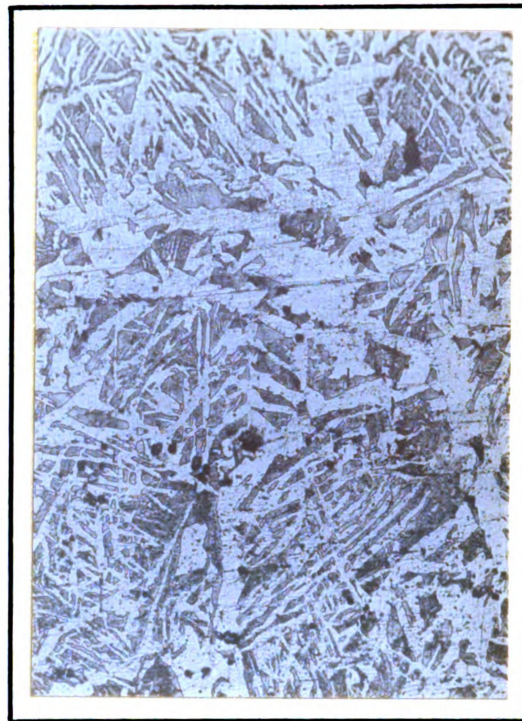
Fig.30. Cooled 1.9 minutes thru critical temperature.
