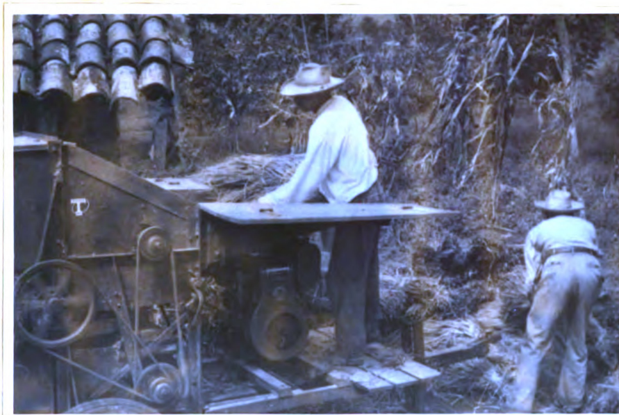
Fig. 11. Stationary threshing machine. Units of this type are now being operated under the supervision of the Extension Service.
