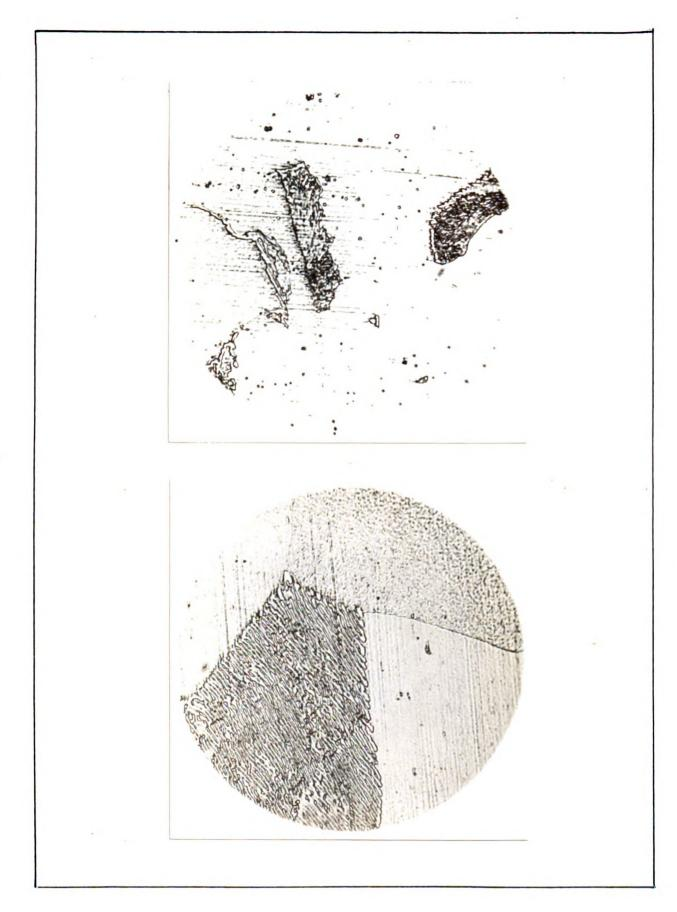
the first water quench, seems to be little affected. However, there is a noticeable less of cementite in the pearlitic areas; the margins in some cases have disappeared and the lamellae have become thinner. Markedly enough, the ferrite has become much disturbed, not being as clean as formerly. The grain boundaries have not increased in size. (Fig. 13)
