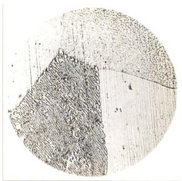
the first water quench, seems to be little affected. However, there is a noticeable less of cementite in the pearlitic areas; the margins in some cases have disappeared and the lamellae have become thinner. Markedly enough, the ferrite has become much disturbed, not being as clean as formerly. The grain boundaries have not increased in size. (Fig. 13)
