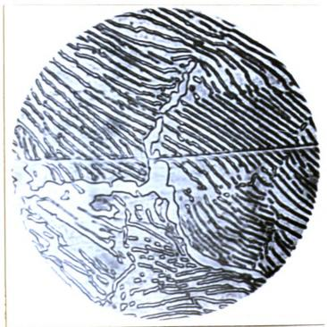
effect upon the ductile properties of steels depending upon the location of the cementite. In order to determine the exact effect these cementite fermations have upon the ductility of low carbon steel, specimens of 5 inch round, 20% carbon, cold rolled steel were prepared in the regular manner for the Isod impact tests. All the pieces were heated in the furnace to 1850°F for one hour. They were then cooled to 1675°F.
