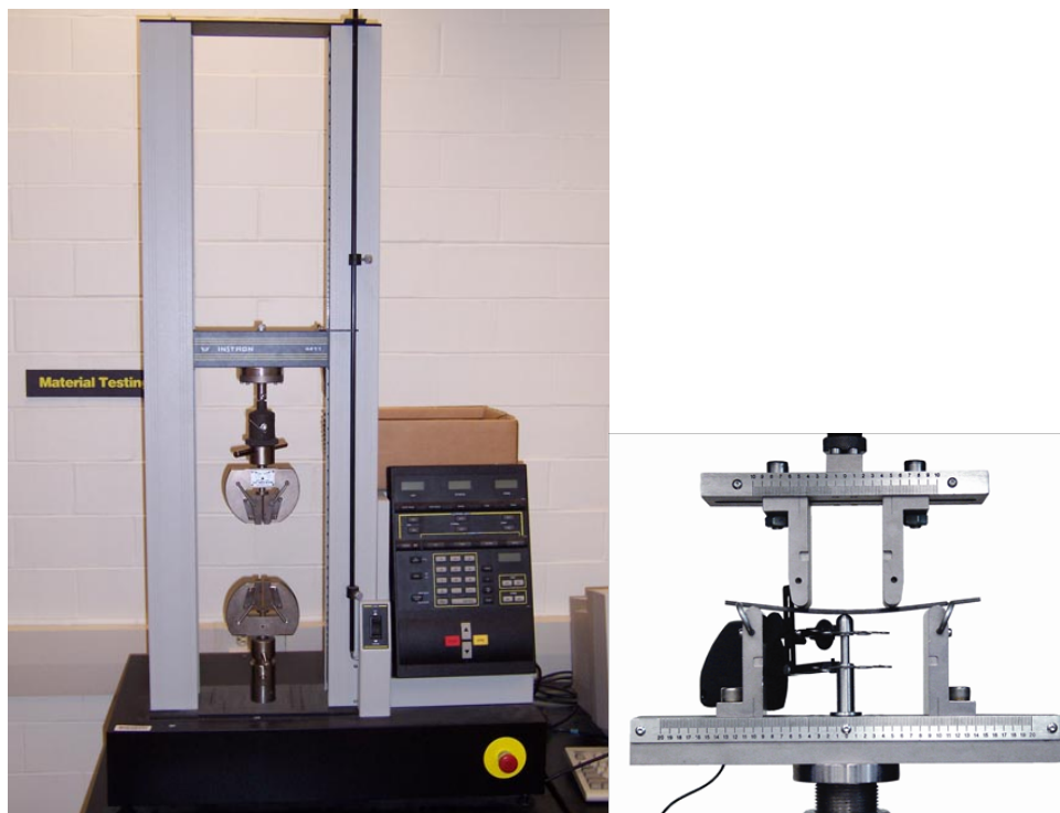
Figure 2.3. An Instron® Universal Machine was used for mechanical testing (left) and can be fitted with a crosshead specific for four-point bending tests (right).
