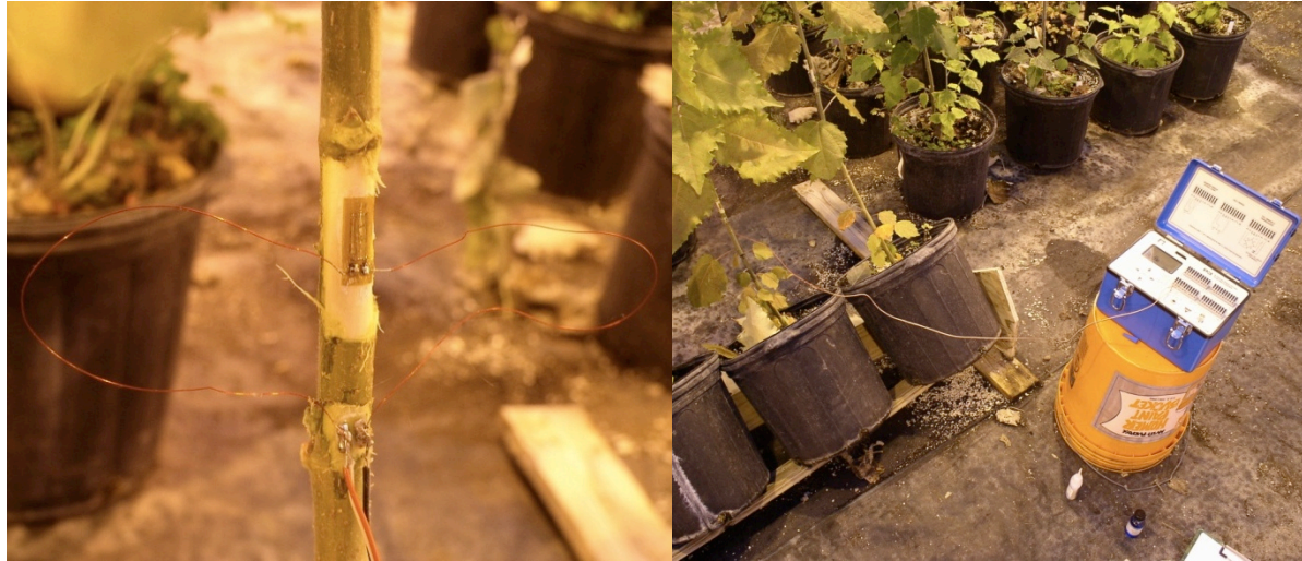
Figure 2.2. (Left) A strain gauge was bonded to the wood surface longitudinally along the grain of inclined hybrid poplar trees that recovered the vertical position. (Right) Released strain was measured every second during the cutting process using a P3 Strain Indicator and Recorder.
