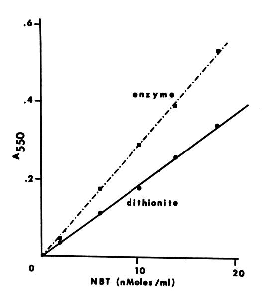
Figure 5. -- NBT diaphorase activity versus protein concentration. Whole goat microsomes were used. The assays were done in 0.05  $\underline{\text{M}}$  Tris-HCl (pH 7.5) with a NBT concentration of 1  $\underline{\text{mM}}$ . Activity is expressed as  $\Delta A_{550}/\text{min}$ .
