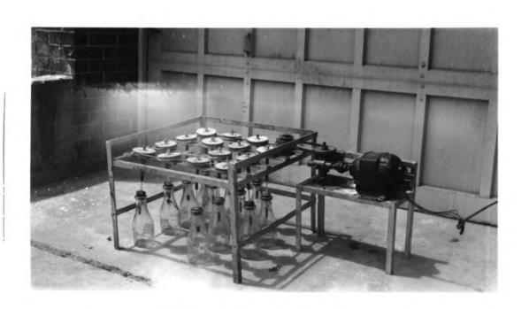
STIRRING APPARATUS USED IN TESTS WITH STEEL RODS
