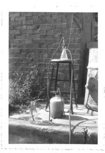
MODEL ZEOLITE SOFTENER USED IN TESTS
