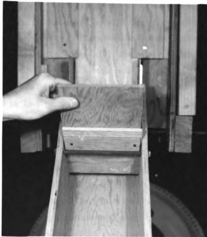
Fig. 4 - A plywood gate was used to control the flow of corn through the chute orifice.
