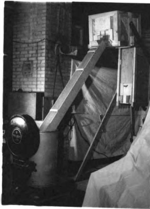
Fig. 5.- Corn flowing from the portable bin through the long wood chute and into the scale bin.
