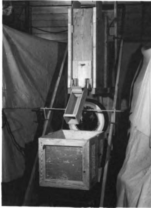
Fig. 1 - An over-all view of the apparatus showing the storage bin, portable bin and platform scales.
