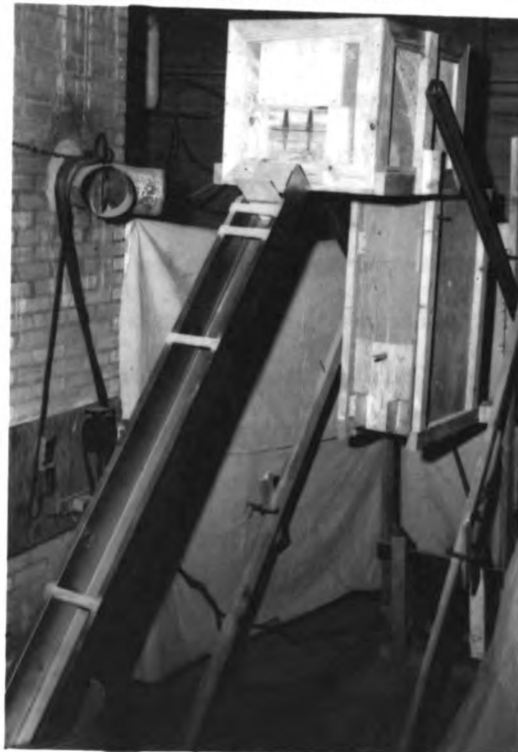
Fig. 6 - A long steel chute mounted to measure the flow rates and the depths of corn flowing in the chutes.
