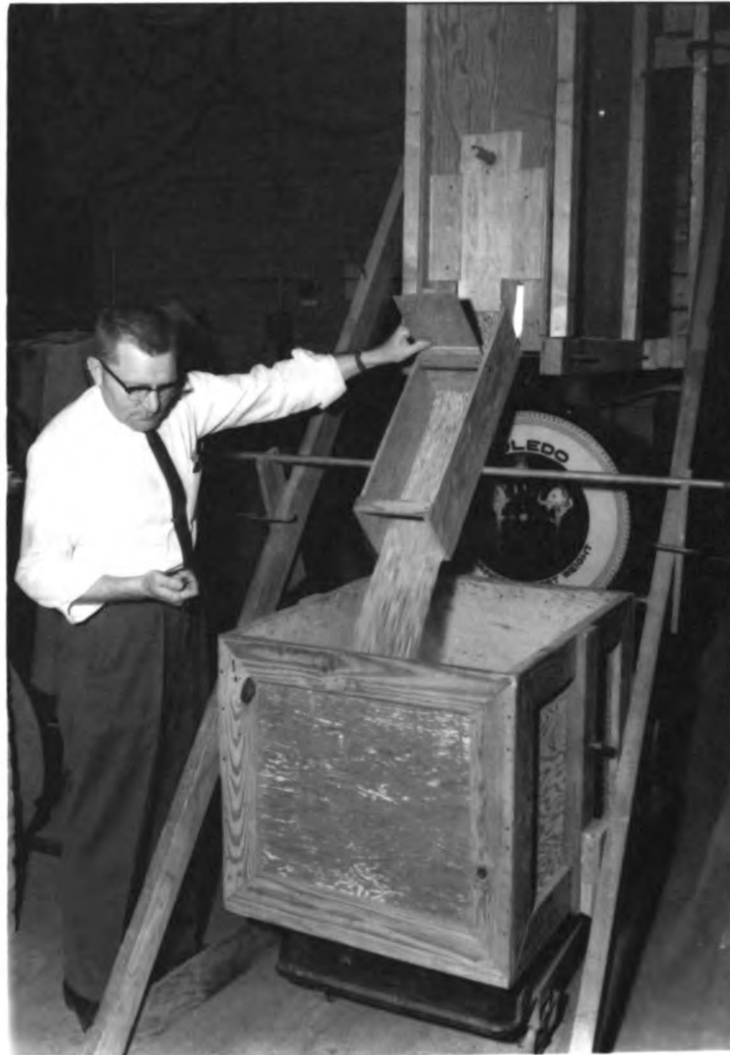
The author is shown timing the rate of flow of shelled corn through a short ( 1\frac{1}{2} ft) wood chute using a 1\frac{1}{2} x 6 in. orifice in the chute.
