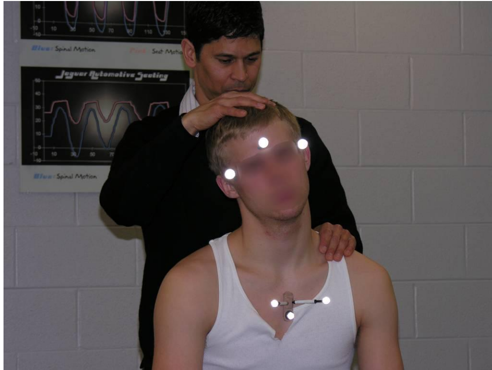
Figure 7. Retro-reflective passive markers applied to the forehead, left and right temple, and a triad configuration on the sternum
