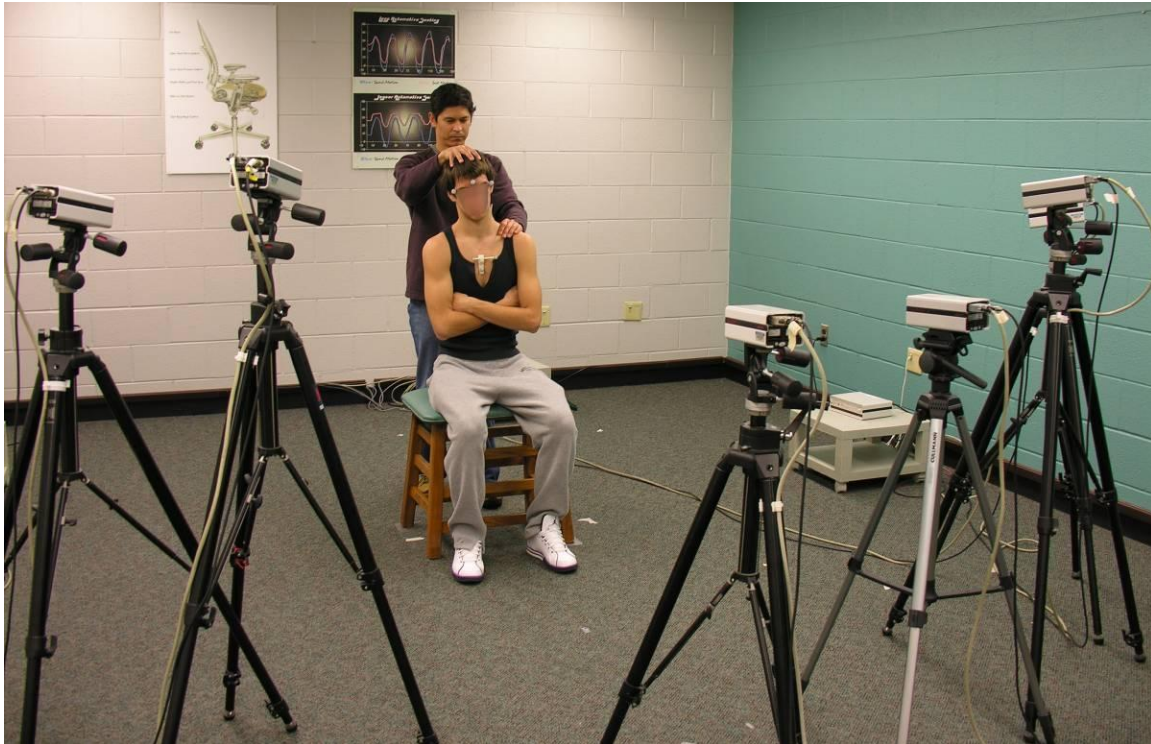
Figure 8. Motion capture system camera configuration with global coordinate system origin on the left, posterior stool corner relative to the subject
