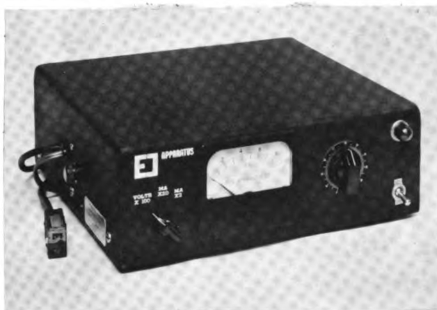
Figure 1a. E-C Power Supply: input 110-120 v.; output adjustable 0-1000 v. at 200 ma. or less; two units can be connected in series for 2000 v. output.
