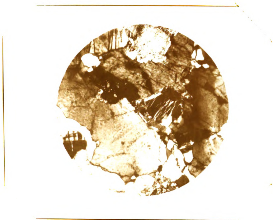
Figure 3. Photomicrograph of sample 21 showing xenomorphic-inequigranular texture of the granite. Crossed nicols, X54 diameters.
