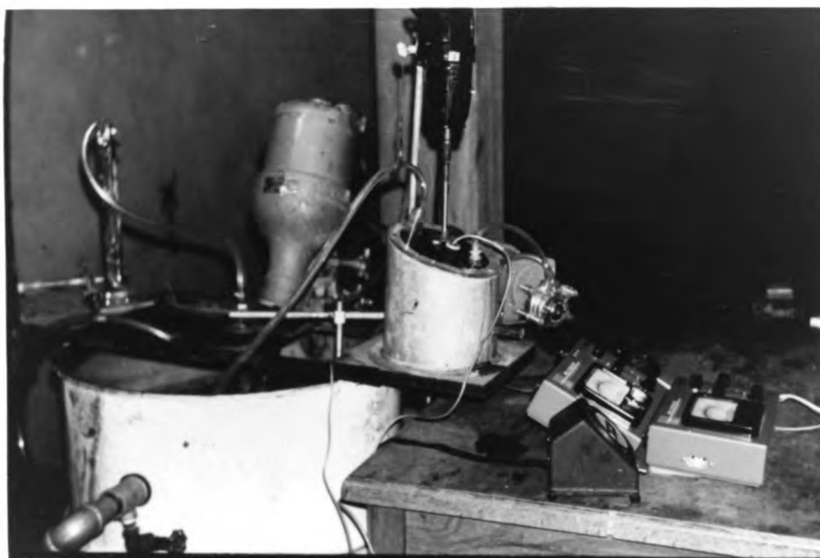
Figure 3. Flow through respirometer attached to continuous flow culture apparatus.
