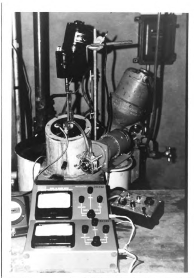
Figure 4. Flow through respirometer showing respiration cell, variable speed peristaltic pump and DO meters.
