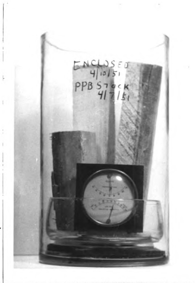
Figure 1. Large battery jar type cage; water; hickory.
