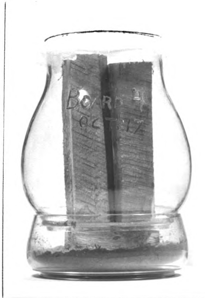
Figure 2. Lamp globe cage with moist sand.
