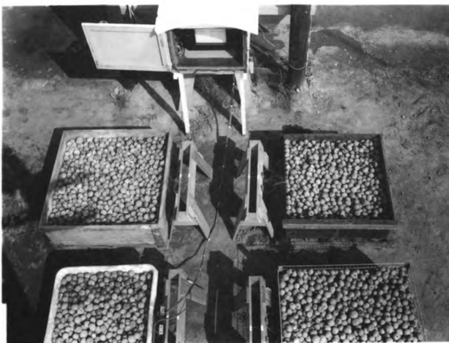
Figure 1. Tomato temperature study showing the four different types of bulk boxes, the potentiometer and lead wires
