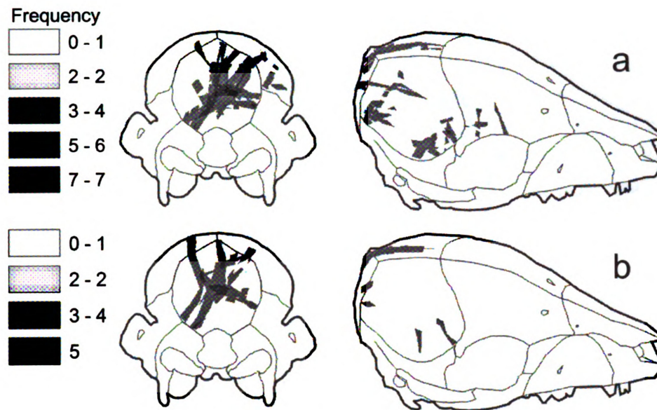
Figure 2.7. GIS map of the 19-28 day old rigid (a) and compliant (b) impacts at high energy.
