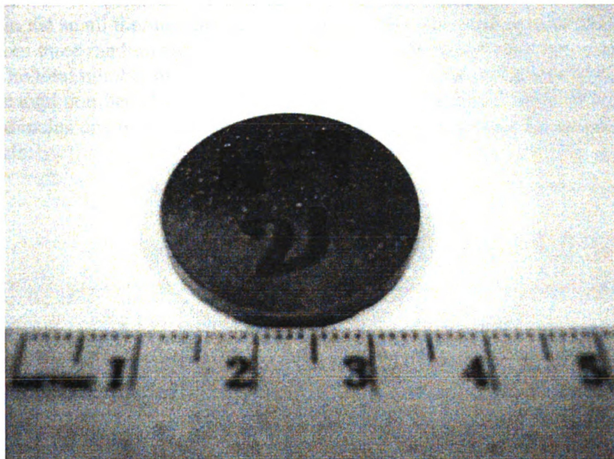
Figure 3.1.2.3b. Surface of LAST specimen N37-21 in contact with the hot plate , showing surface pitting and inclusions after 200 thermal cycles.
