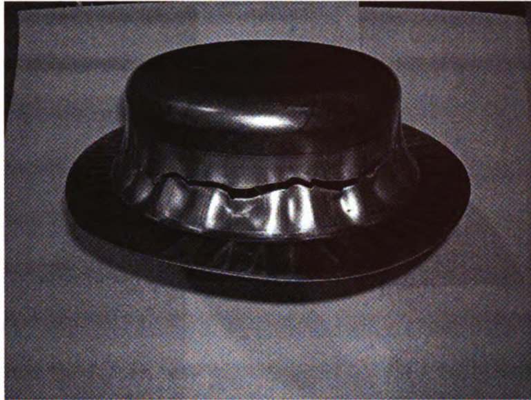
Figure 13 - hydro forming of an 11 in blank with a variable Pressure and a constant BHF.
