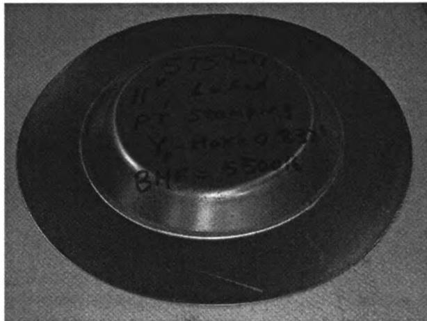
Figure 8: Stamping of 5754-O Aluminum sheet with out pressure with 11 in blank
