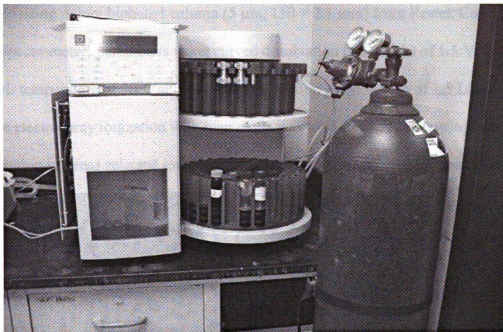
Figure 3.4 Accelerated Solvent Extractor Used in the Experiment
