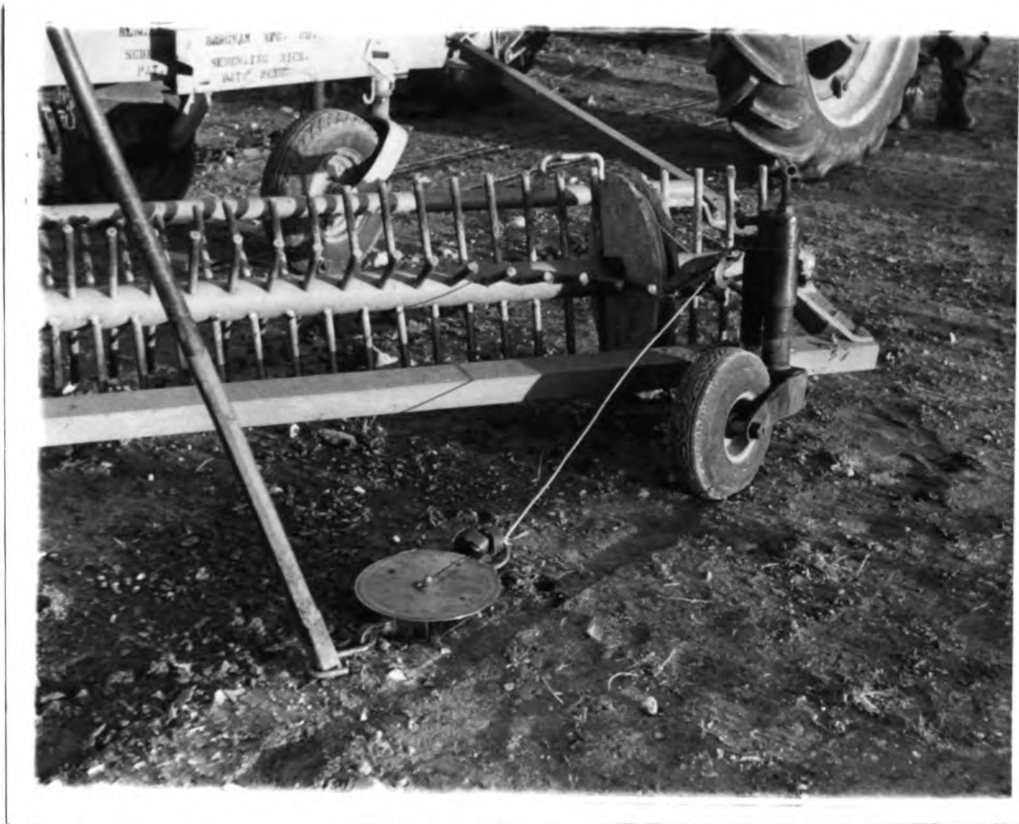
Figure 17. Special drum mounted on windrower shaft for making torque determinations.
