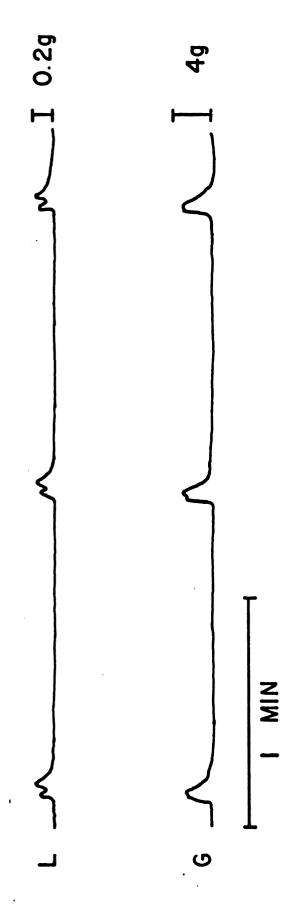
2. The Grass FT-03 transducer showed a contraction peak while the longitudinally oriented extraluminal transducer showed an initial contraction peak, and then a slight relaxation followed by another contraction peak.
