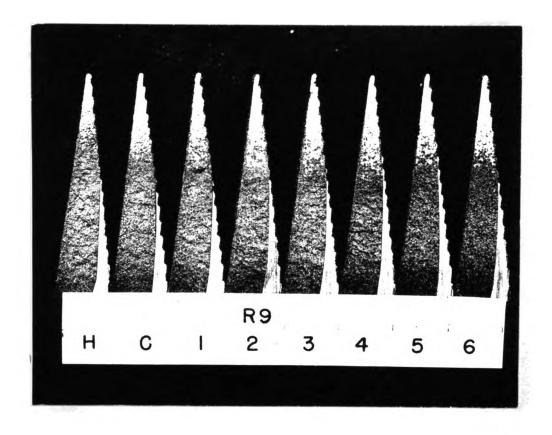
Figure 14. Effect of pouring temperature and holding time on chilling tendency of uninoculated cast iron (Heat R9).
