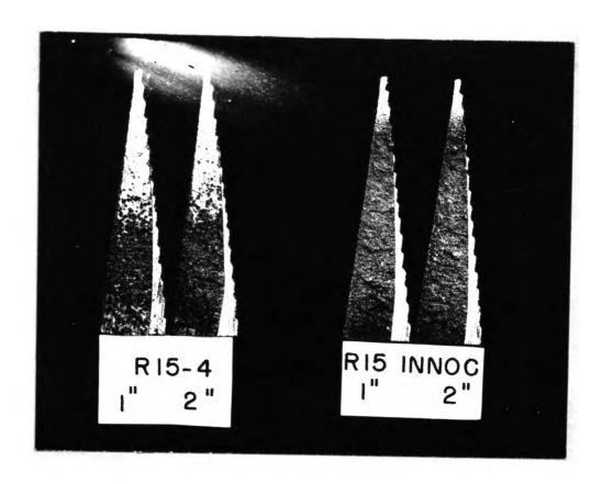
Figure 5. End cooling effect on chill depth for wedge test.
