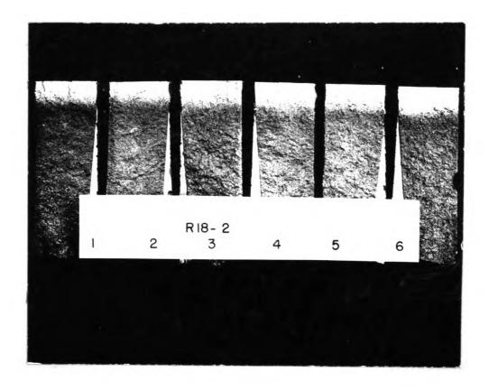
Figure 10. Effect of pouring rate on chill depth of horizontal chill block test poured from inoculated cast iron.
