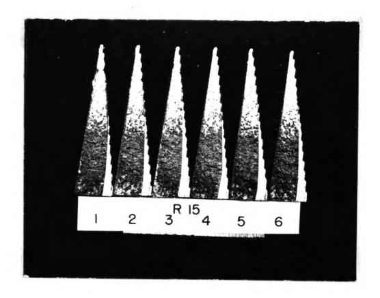
Figure 1. Consistency of wedge chill tests poured from uninoculated cast iron.
