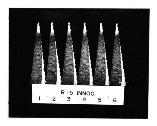
Figure 3. Consistency of wedge chill tests poured from inoculated cast iron.
