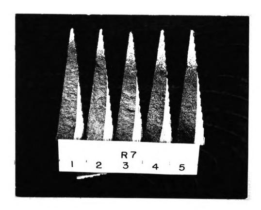
Figure 12. Effect of pouring temperature and holding time on chilling tendency of inoculated cast iron (Heat R7).
