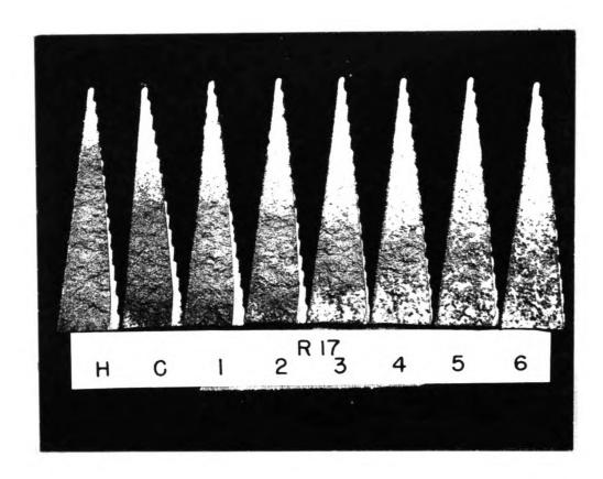
Figure 18. Effect of holding time and pouring temperature on chilling tendency of inoculated cast iron (Heat R17).
