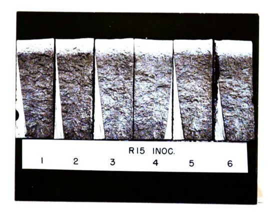
Figure 4. Consistency of chill block tests poured from inoculated cast iron.
