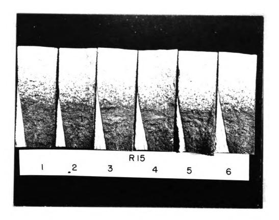
Figure 2. Consistency of chill block tests poured from uninoculated cast iron.
