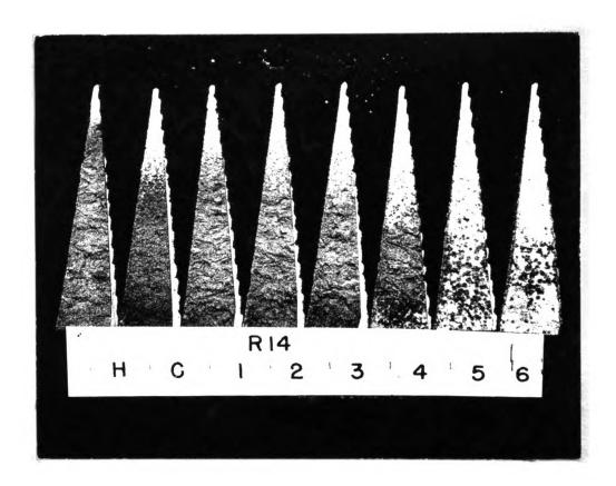
Figure 17. Effect of holding time and pouring temperature on chilling tendency of inoculated cast iron (Heat R14).
