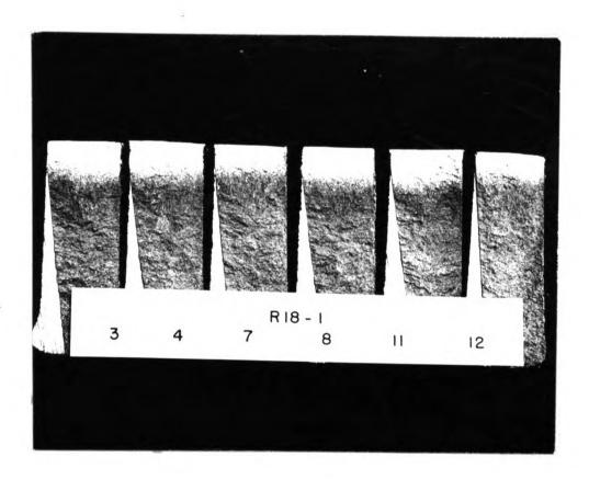
Figure 9. Consistency of horizontal chill block test poured from inoculated cast iron.
