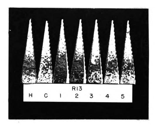
Figure 16. Effect of holding time and pouring temperature on chilling tendency of uninoculated cast iron (Heat R13).
