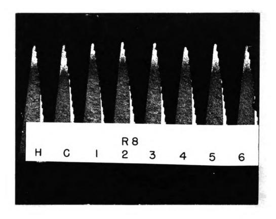
Figure 13. Effect of pouring temperature and holding time on chilling tendency of inoculated cast iron (Heat R8).
