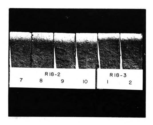
Figure 11. Effect of pouring rate on chill depth of vertical chill block test poured from inoculated cast iron.
