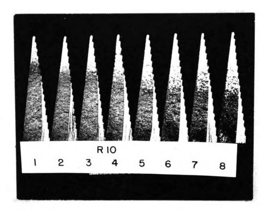
Figure 15. Effect of melting conditions on chilling tendency of uninoculated cast iron.
