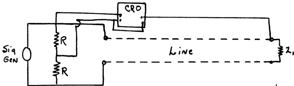
Circuit for Phase Shift Measurements
