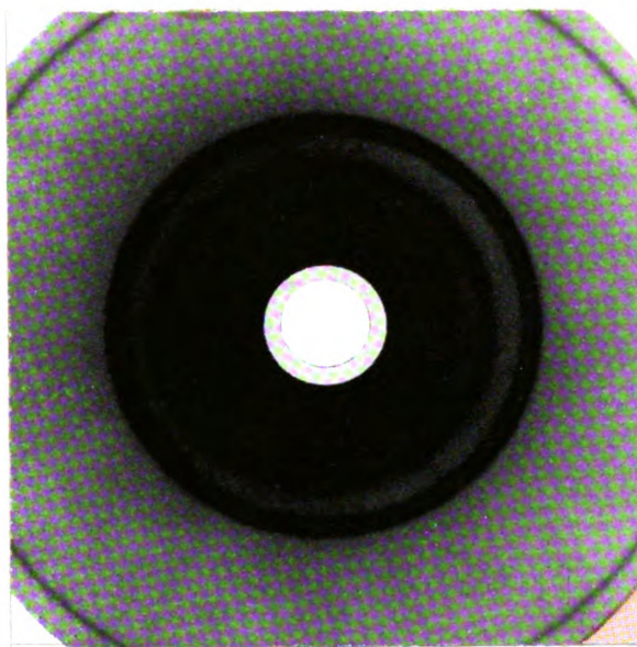
Fig. 16c. Diffraction rings of back reflection photograph.
