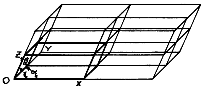
Fig. 1. The crystal space-lattice.
