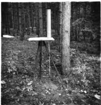
FIGURE 5: Apparatus used in making crown density measurements.
