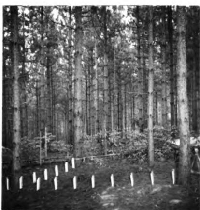
FIGURE 7: Rain gauges radiating from a central tree to neighbouring trees.
