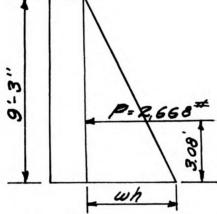
Total Pressure on wall from sewage (per foot length of wall).
