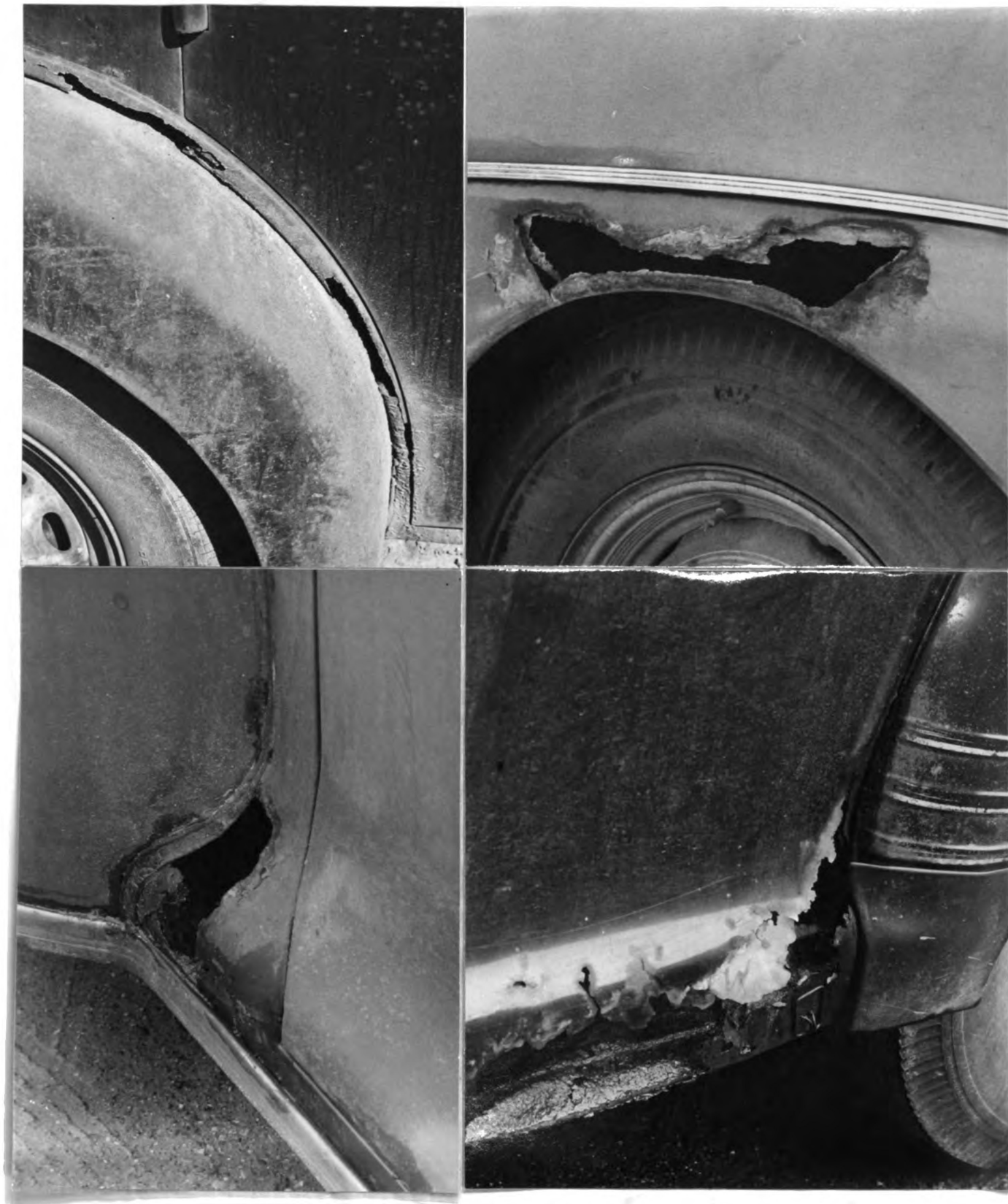
Figure 1. Typical examples of the corrosion of automobile bodies.
