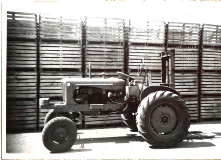
Figure 36. Field lift tractor. This tractor has been rebuilt for use in the muck fields. It is designed to lift the crates in the background.
