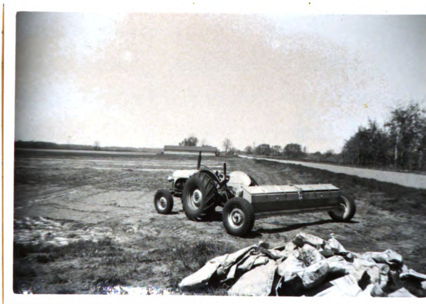
Figure 36. Field lift tractor. This tractor has been rebuilt for use in the muck fields. It is designed to lift the crates in the background.
