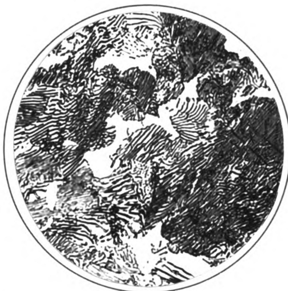
Figure 47 Eutectoid Zone Carburized 3 Hours at 1700°F. Mag. 1000X
