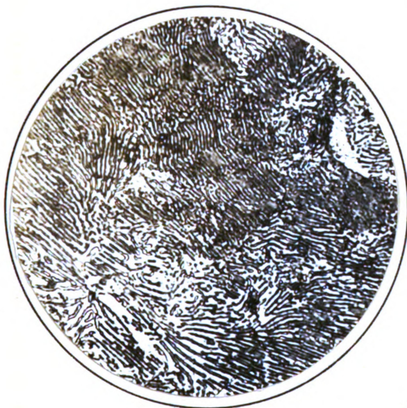
Figure 45 Eutectoid Zone Case Carburized 8 Hours at 1700°F. Mag. 1000X
