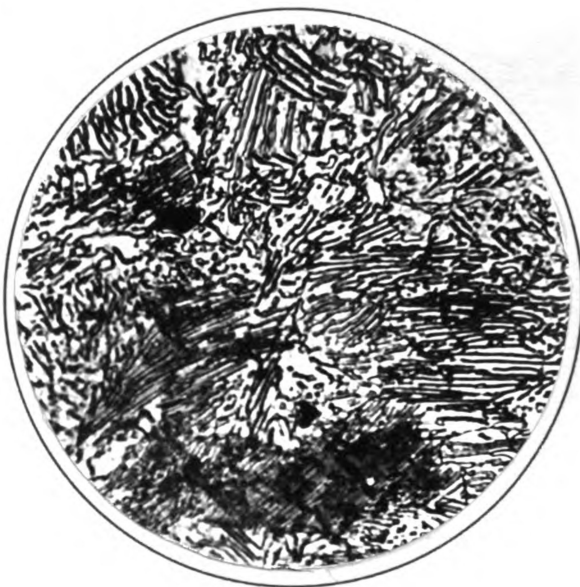
Figure 49 Eutectoid Zone Carburized 1 Hour at 1700°F. Mag. 1500X
