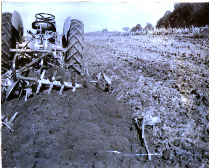
Fig. 4. Courey's short-toothed tiller mounted on the 'Z' hitch.
