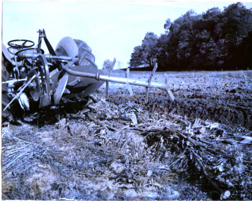
Fig. 6. Courey's long-toothed tiller shown in the elevated position when lifted with the plow.
