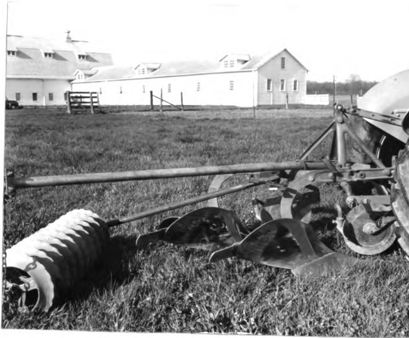
Fig. 8. The cultipacker unit used with the 'L' hitch shown when on the ground.
