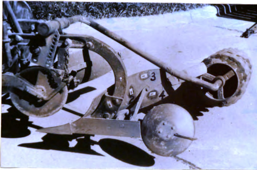
Fig. 19. Positions of the gages on the rear plow-bottom.
