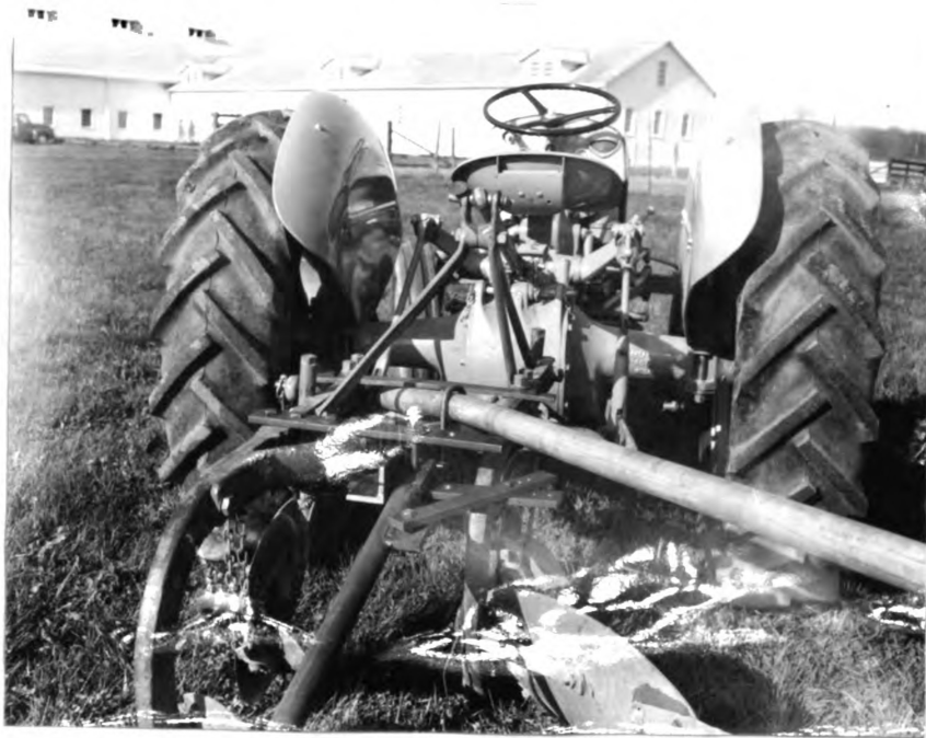
Fig. 11. A view of the hitch bar and direction lever of the 'L' hitch, and the boom support on the plow beam.
