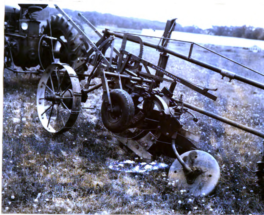
Fig. 17. View showing the plow tipping when the packer was attempted to be lifted.
