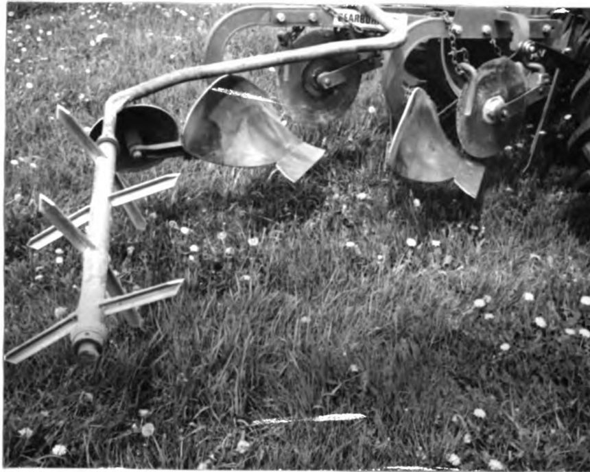
Fig. 5. Courey's long-toothed tiller mounted on the 'Z' hitch.
