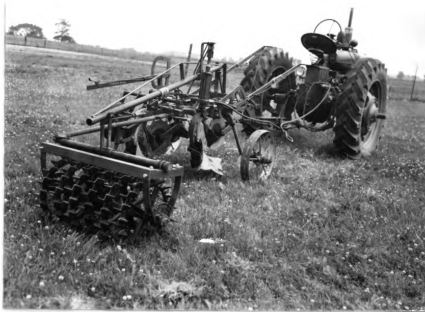
Fig. 15. The plow-packer unit used with the 'L' hitch in tandem with a trail-type plow. Note the boom and hydraulic cylinder used for lifting.
