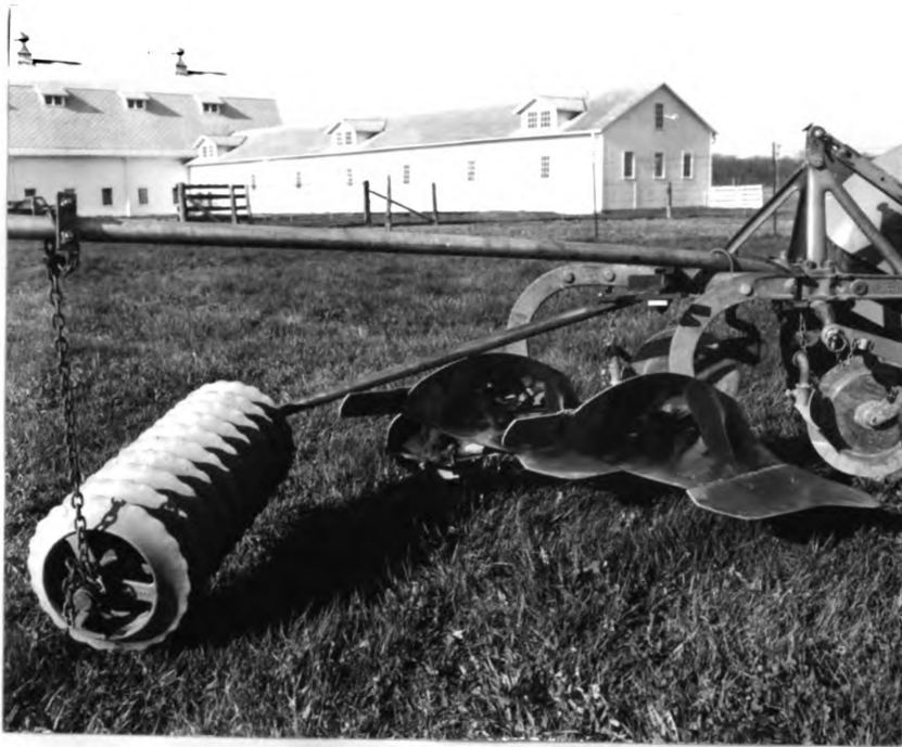
Fig. 10. The cultipacker unit lifted off the ground. Note the outer end of unit is supported by chain clamped to boom.
