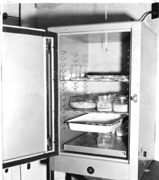
Fig. 2. Interior view of incubators used for rearing the test insects, and as recovery cabinets.
