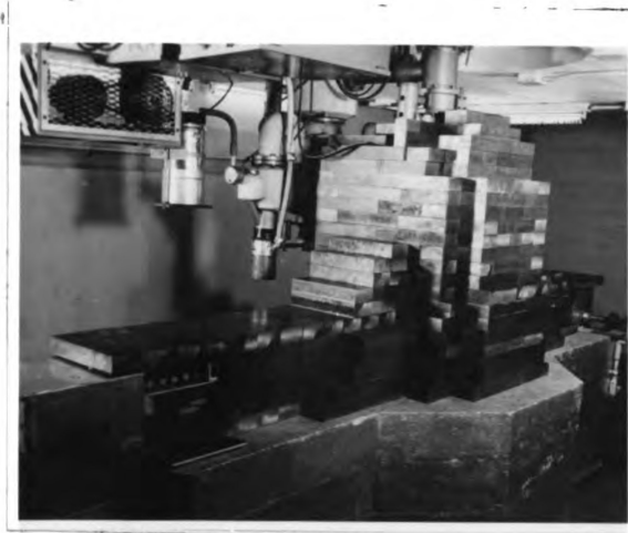
Fig. 10A. View of conveyor belt, shielding blocks and vacuum pump for the Van de Graaff generator. Picture courtesy of the Upjohn Company.
