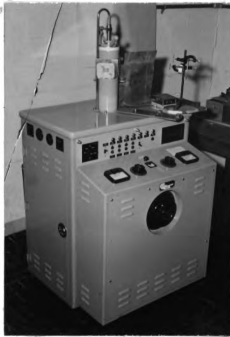
Fig. 9A. General view of the 50 KV Hilger machine used for the x-ray tests.
