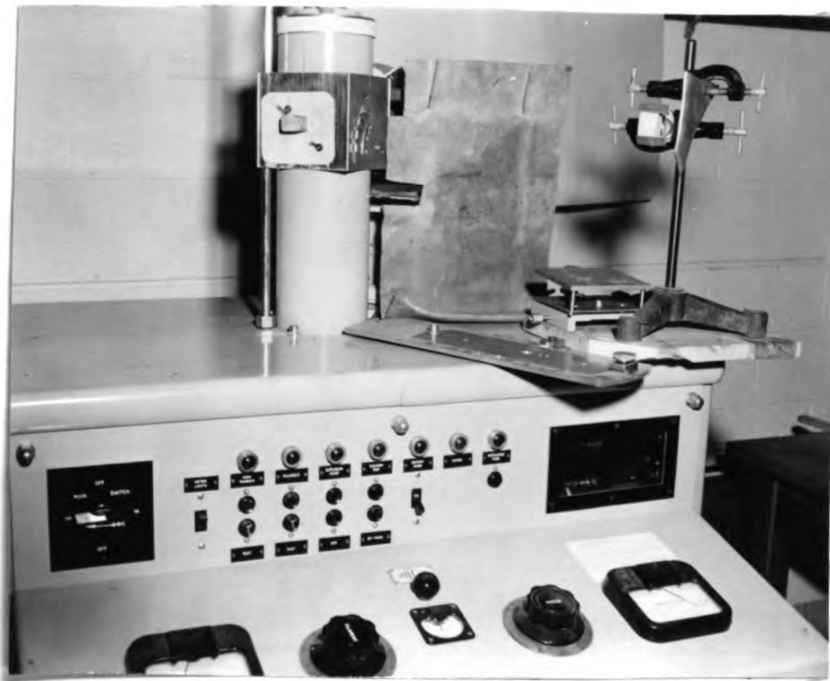
Fig. 9B. Close up view of controls for the Hilger machine. A test sample may be seen in the upper right part of the picture.
