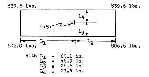
To test the car, there must be a driver added to above weight of the car.
