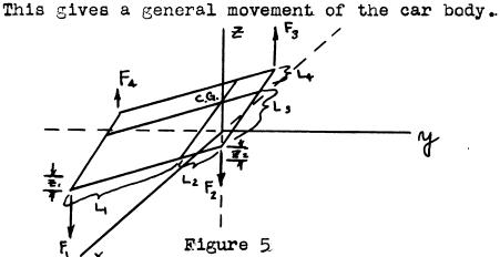
With the forces and displacements upward considered positive, the equations for the above general motion are::
