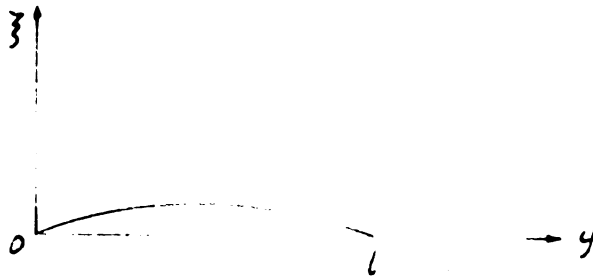
Fig. 1 A bowed-out dislocation
