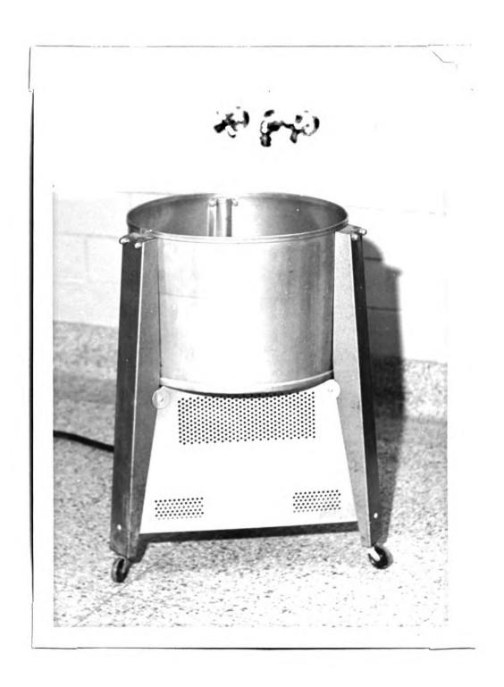
FIGURE I. Keenco Egg Washer Model 750. Air-Jet Action. Washer A, manufactured by Keen Manufacturing Company, Vineland, New Jersey.
