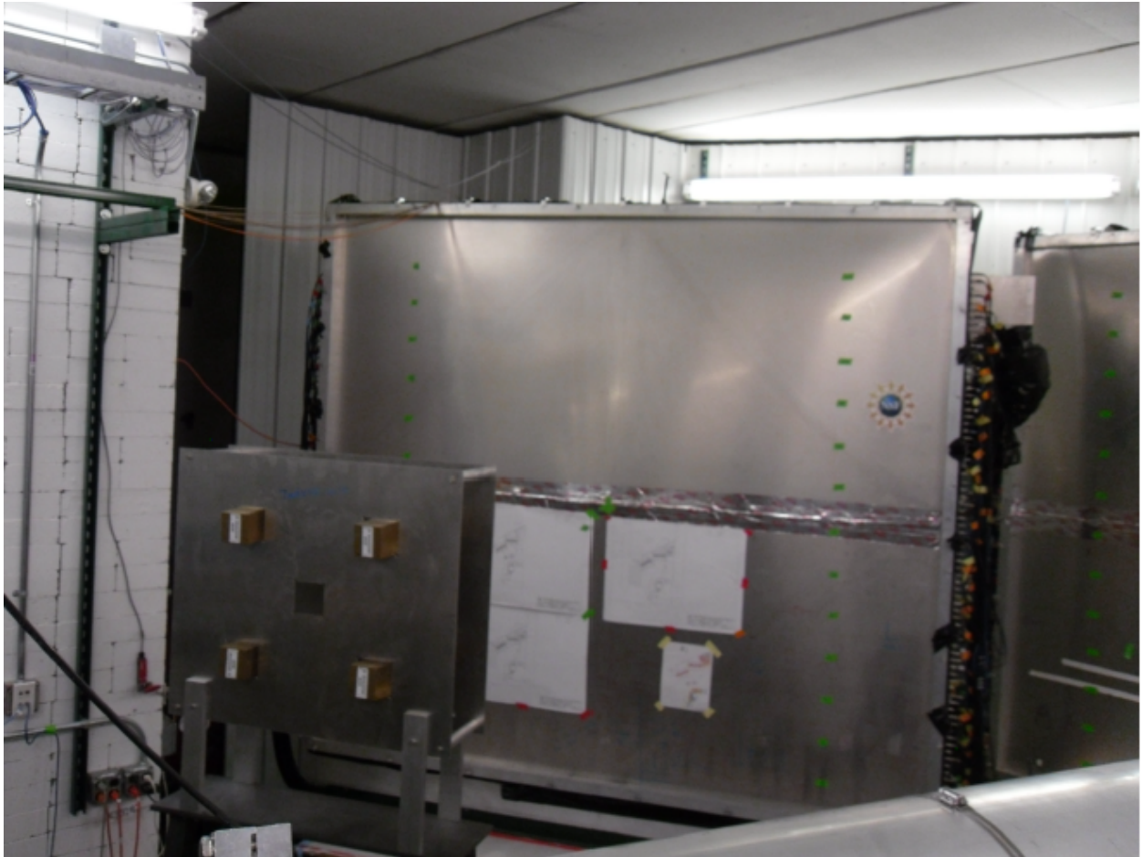
Figure 3.10: Four shadowbars in one of the configurations used in the experiment.
