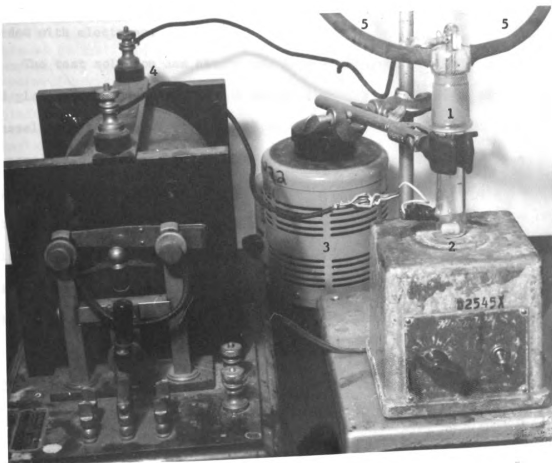
Figure # 11- Experimental Setup 1: Reaction chamber 2: Magnetic stirrer 3: Power supply 4: Induction coil 5: Ventilation
