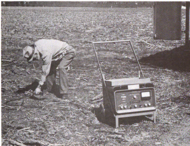
Figure 8. Operator placing gamma-ray surface density gage for field determination of soil density.
