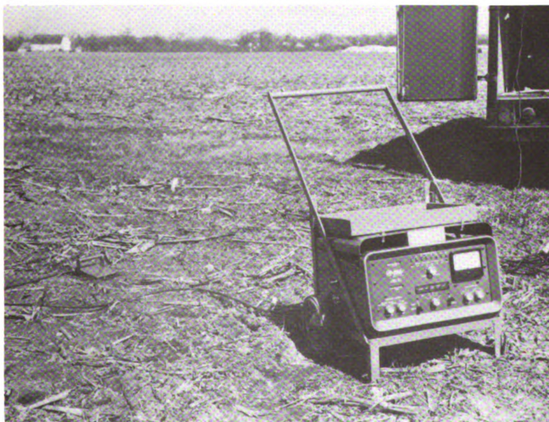
Figure 9. Gamma-ray surface density gage in use for field determination of soil density.
