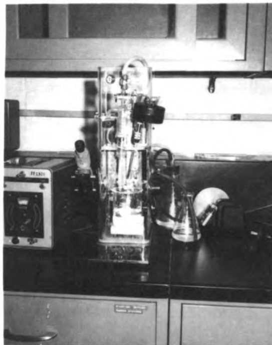
Figure 8. The Coulter Counter Industrial Model B. Above: (a) General view of Coulter Counter. Below: (b) Close-up of aperture tube stand.
