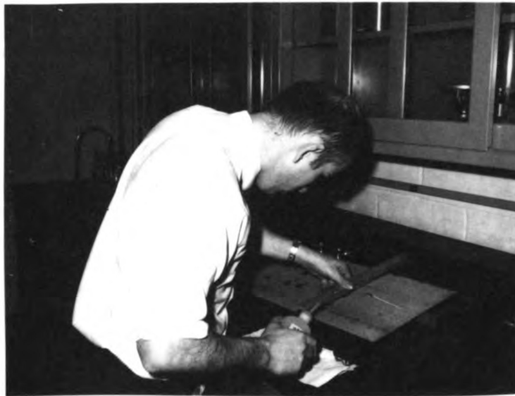
Figure 5. Photographs of experimental stage of study. Above: (a) General view of apparatus used in the study. Below: (b) Removal of sample from bed plate. Note position of squeegee and use of wash- bottle.
