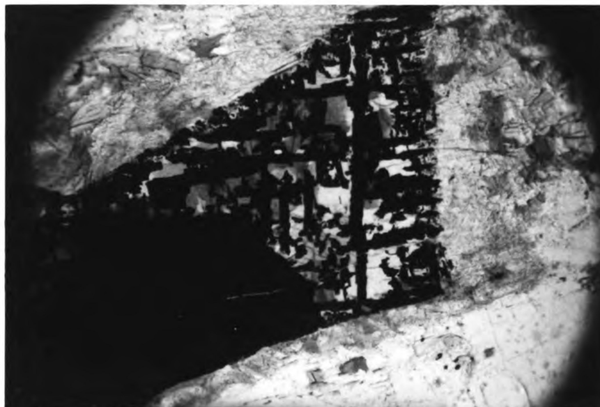
Figure 20 Photomicrograph of 32-66 illustrating magnetite skeleton left after ilmenite has been eaten away in plain light X 80 diameters.
