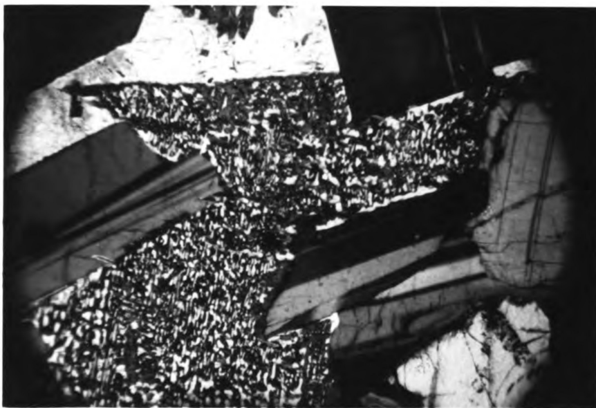
Figure 26 Photomicrograph of 32-61 illustrating pigeonite-augite exsolution. Crossed niccols.
