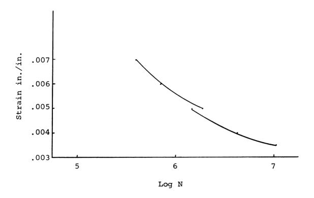
Figure 11. Strain amplitude vs. log of number of cycles for failure -- annealed copper.
