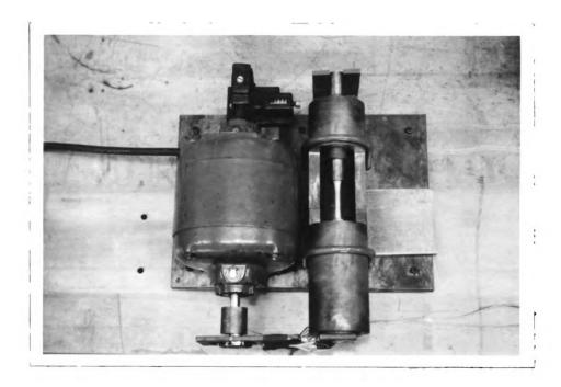
Figure 3. Constant strain amplitude torsional fatigue machine, top view.
