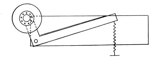
Figure 1. Constant load burnishing tool.
