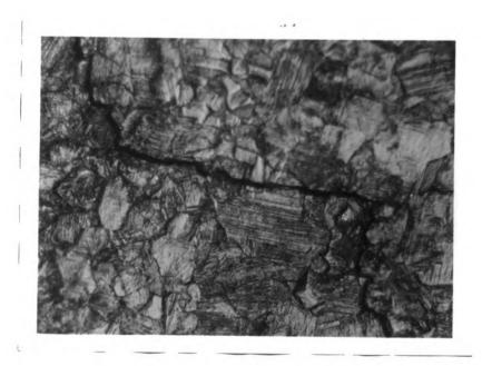
Figure 10. Fatigue crack in annealed copper at 0.004 in./in. strain. 570x.
