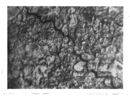
Figure 8. Fatigue crack in annealed copper at 0.005 in./in. strain, high strain mode. 570x.
