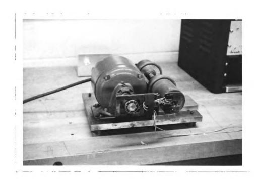
Figure 2. Constant strain amplitude torsional fatigue machine, front view.
