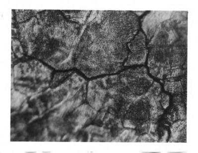
Figure 6. Fatigue crack in annealed copper at 0.007 in./in. shear strain. 570x.
