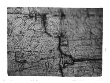
Figure 14. Fatigue crack in burnished copper. 570x.
