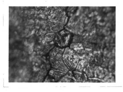
Figure 7. Fatigue crack in annealed copper at 0.006 in./in. strain. 570x.
