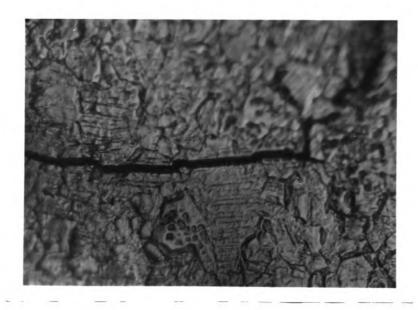
Figure 9. Fatigue crack in annealed copper at 0.005 in./in. strain, low strain mode. 570x.
