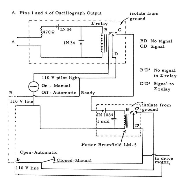
Figure 4. Circuit diagram for the automatic shut-off relay system.
