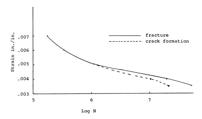
Figure 13. Strain amplitude vs. log of number of cycles for crack formation and fracture -- burnished copper.
