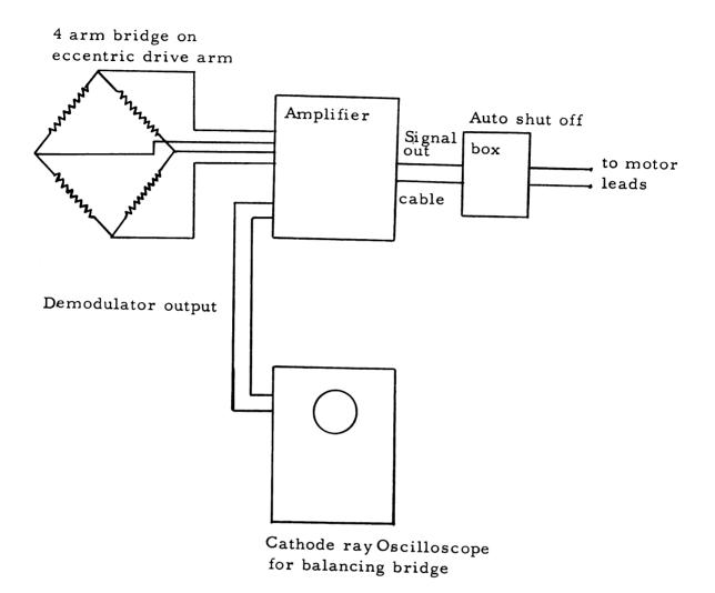
Figure 5. Assembly of the automatic shut-off relay system with the bridge circuit.
