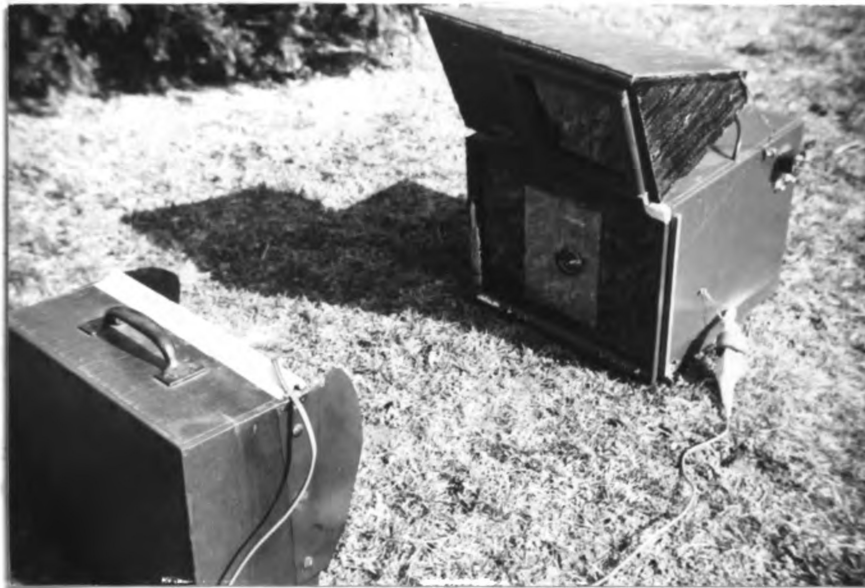
Plate 2. A front view of the camera box showing the camera within and the flash unit mounted above. (Note: the photographs of the apparatus were not taken to show the environmental placement.)
