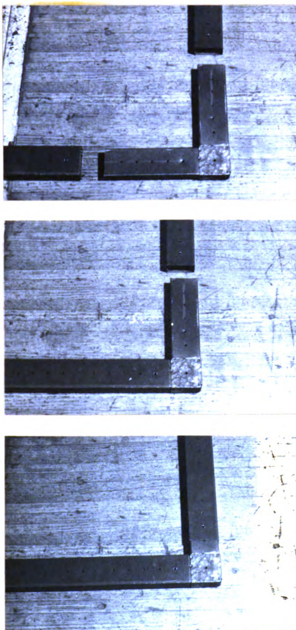
Figure 13. Insertion of corner piece into rail and stile.
