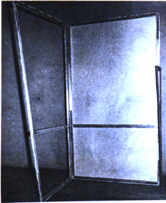
Fig. 21. Prefabricated aluminum book-flat. This photograph illustrates the need for more internal bracing than that furnished by a single toggle. The flat on the right is supported by a rectangular wood brace.
