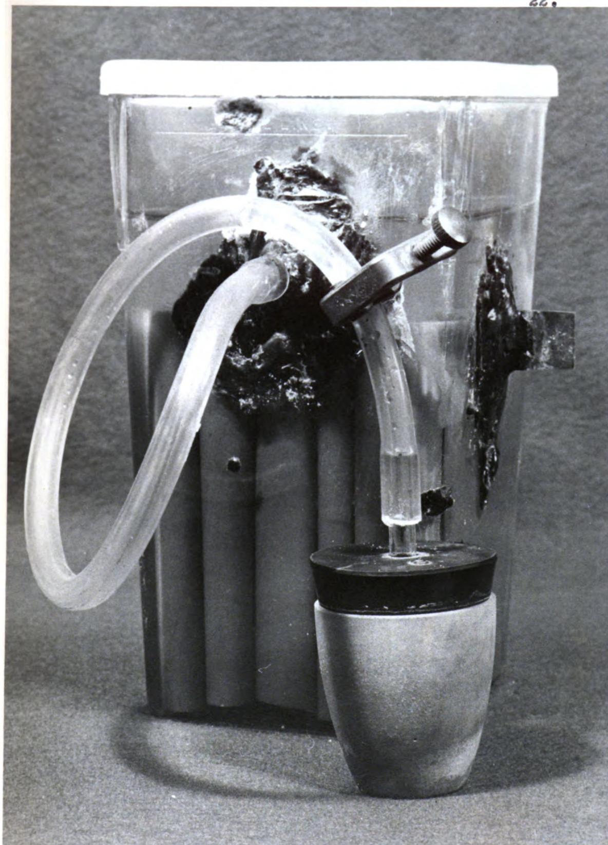
FIGURE 5: Standard Silver-Silver Chloride Reference Electrode, Side View
