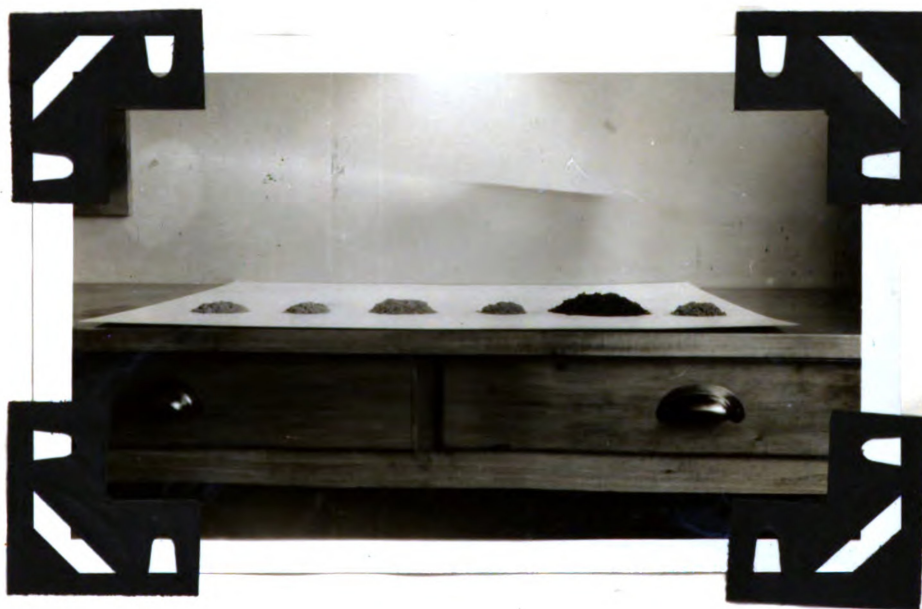
MINERAL MATTER IN THE FIBROUS MATERIAL - From left to right:- TYPE "B", HOOSIER FIBROUS, MEADOWS FIBROUS, "WEBBED", JOHNS - MAN- VILLE FIBROUS, and "FELT SIDE"
