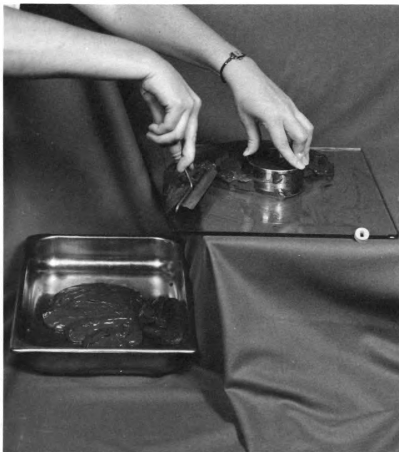
Figure 6. Removing the excess filling from the outer edge of the sample cutter.
