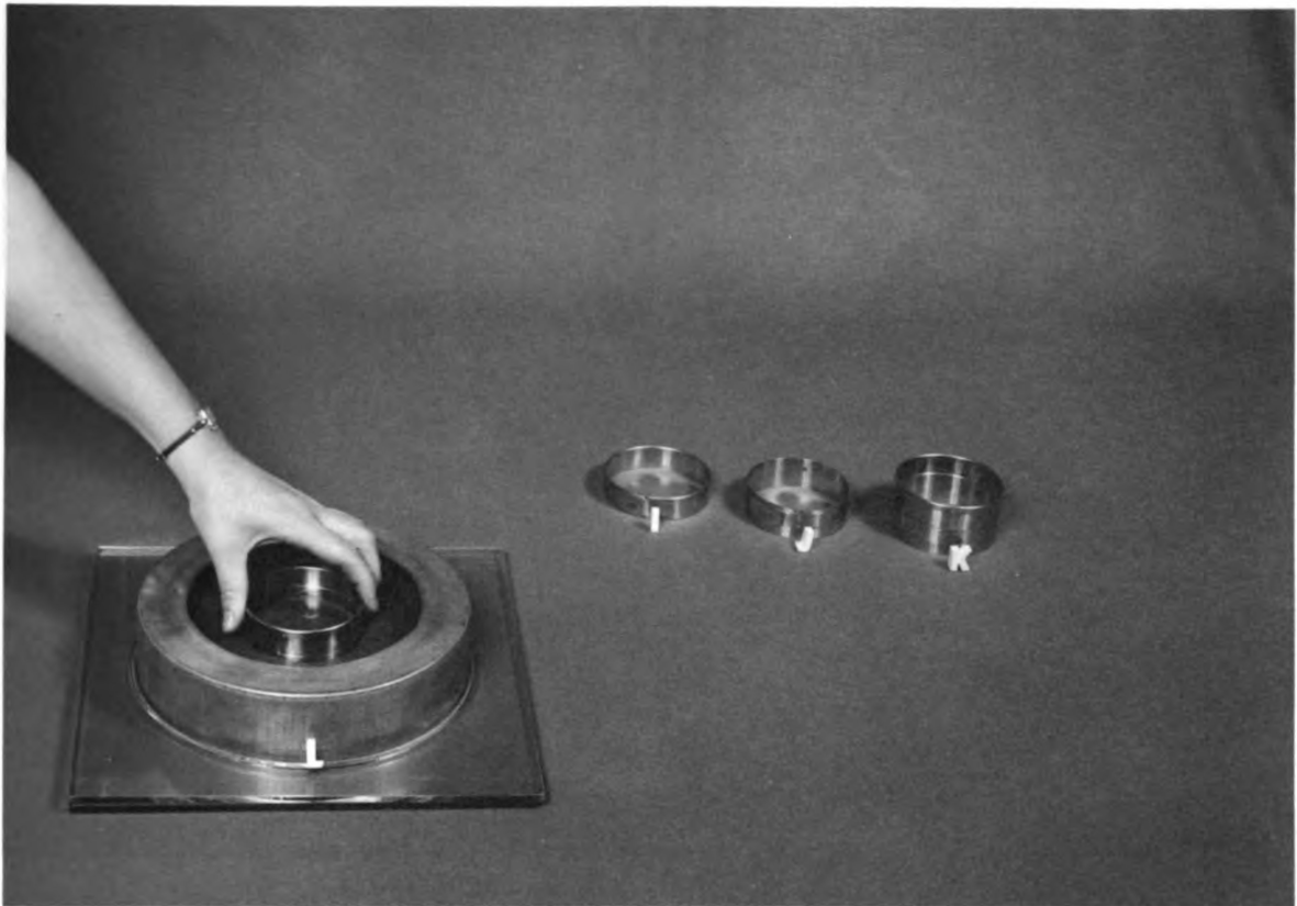
Figure 3. Inserting the sample cutter. Individual parts and complete assembly of sample cutter.
