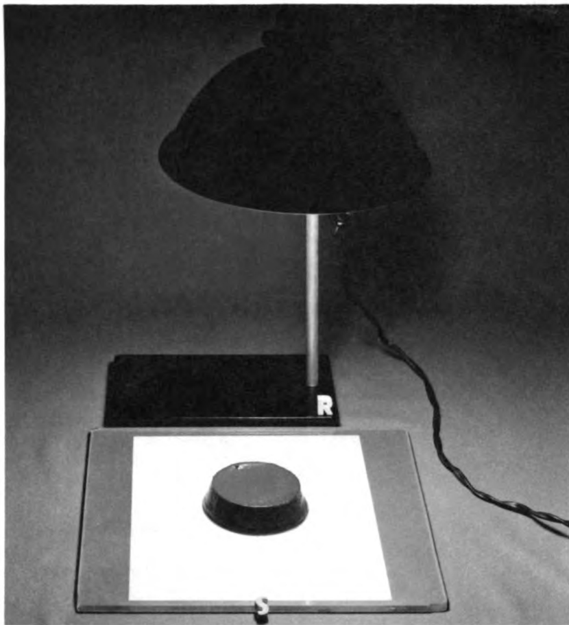
Figure 9. Recording the sample area on Technifax Diazo blue line paper.
