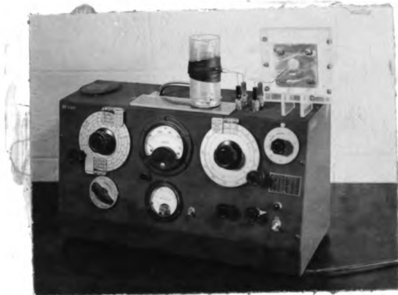
Figure 4. The Boonton 160A "Q" Meter with empty test condenser and inductance connected.
