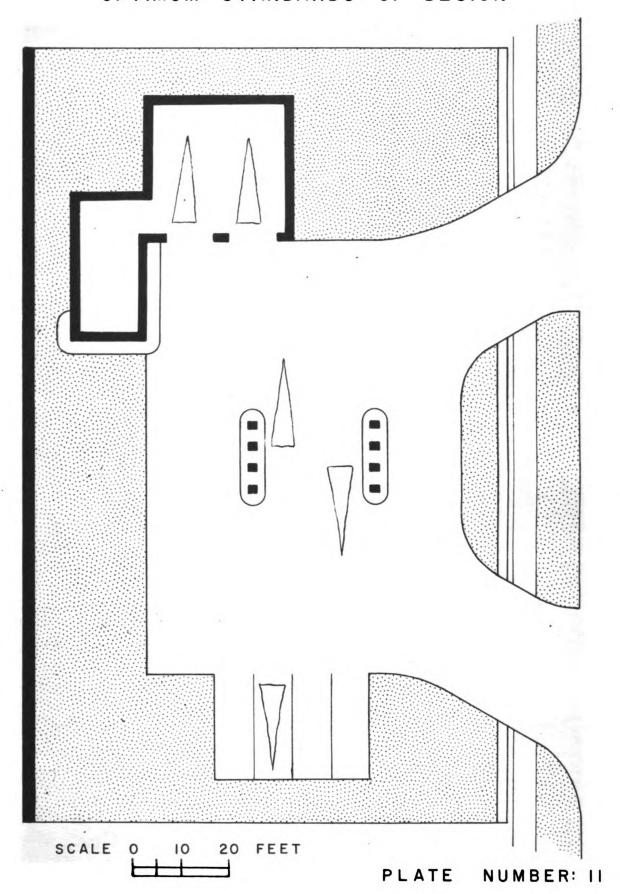
All other standards are carried over from the 'minimum' design, including the requirement for a raised curbing along the street property line, the masonry wall separating the site from residential areas, and the sliding scale by which the size of the service station may be increased.
