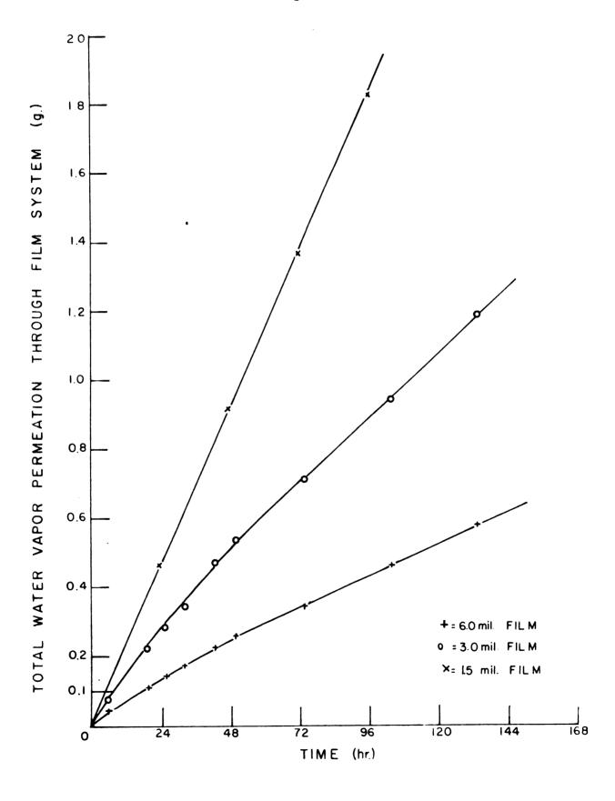
Fig. 4 -- The total water vapor permeation through three different free film thicknesses of the long oil linseed pure alkyd paint (paint no. 2) plotted versus the elapsed time.
