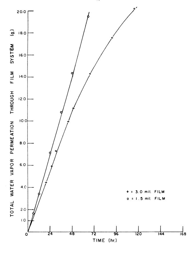
Fig. 7 -- The total water vapor permeation through three different thicknesses of the linseed oil paint (paint no. 1) on the standard redwood substrate plotted versus the elapsed time.
