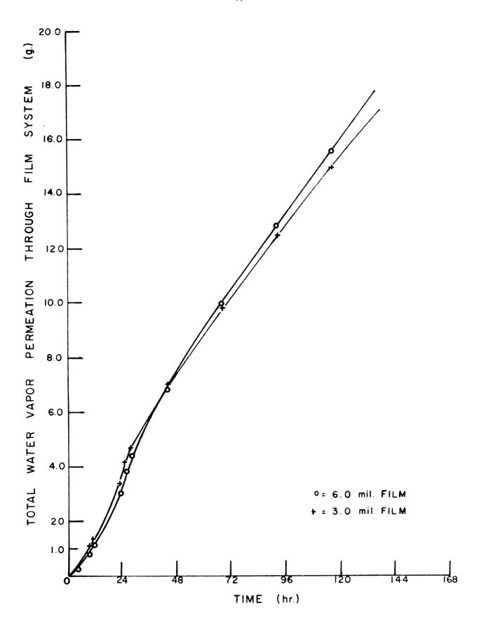
Fig. 10 -- The total water vapor permeation through 3.0 mil. films of the acrylic emulsion paints (paints nos. 4 and 5) on the standard redwood substrate plotted versus the elapsed time.
