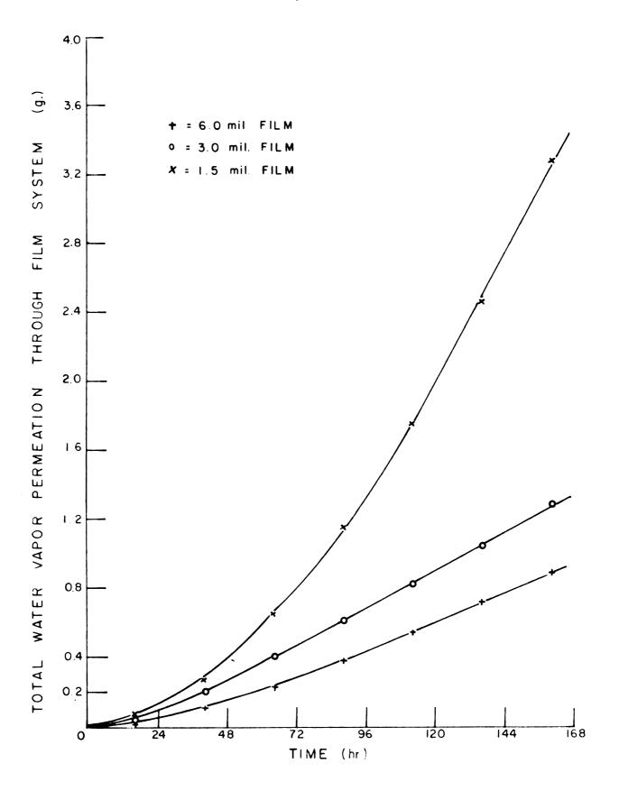
Fig. 5 -- The total water vapor permeation through two different free film thicknesses of the one coat latex paint (paint no. 3) plotted versus the elapsed time.
