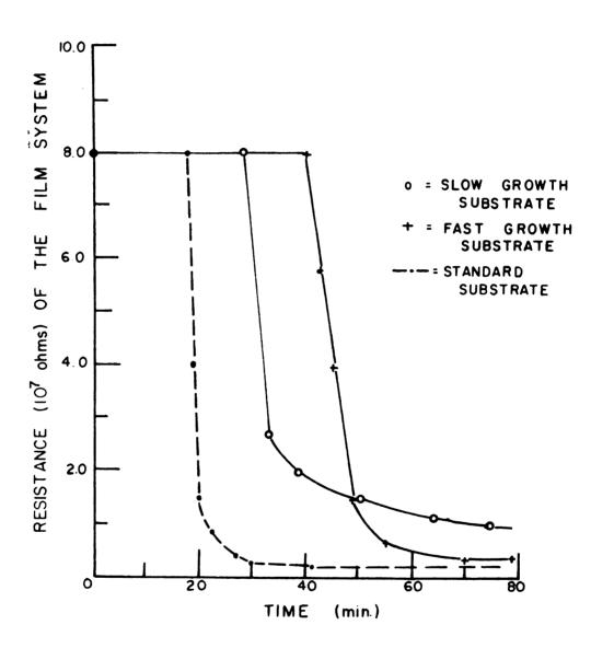
Fig. 23 -- The total liquid water permeation through 3.0 mil. films of the one coat latex paint (paint no. 3) on sanded and steamed substrates was indicated by the resistance decrease plotted versus the elapsed time. The permeation through the standard system was plotted for comparison.
