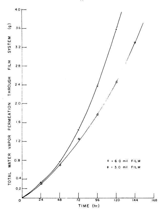
Fig. 9 -- The total water vapor permeation through two different thicknesses of the one coat latex paint (paint no. 3) on the standard redwood substrate plotted versus the elapsed time.
