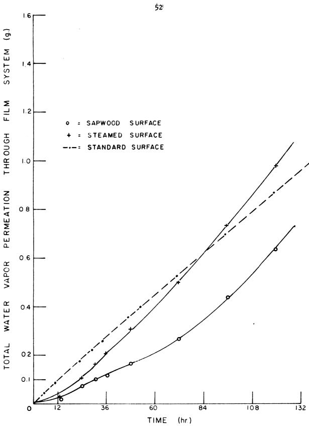
Fig. 13 -- The total water vapor permeation through 3.0 mil. films of the linseed oil paint (paint no. 1) on sliced redwood veneer and planed hemlock plotted versus the elapsed time. The permeation through the standard system was plotted for comparison.
