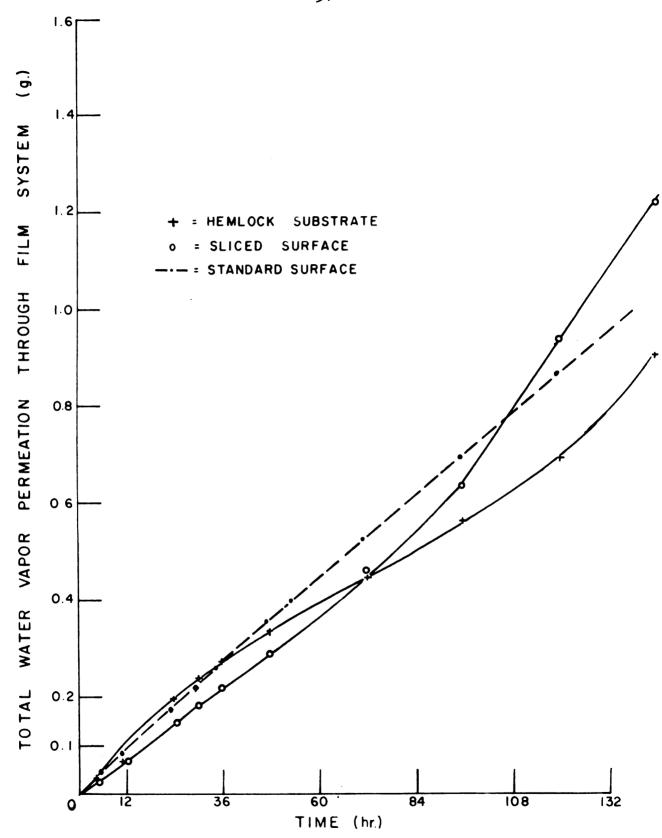
Fig. 14 -- The total water vapor permeation through 3.0 mil. films of the linseed oil paint (paint no. 1) on edge grain, fast growth substrates and inverted standard substrates plotted versus the elapsed time. The permeation through the standard system was plotted for comparison.
