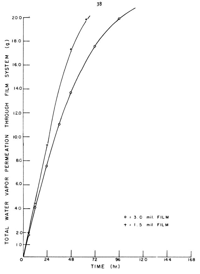
Fig. 6 -- The total water vapor permeation through two different free film thicknesses of the acrylic emulsion paint (paint no. 5) plotted versus the elapsed time.
