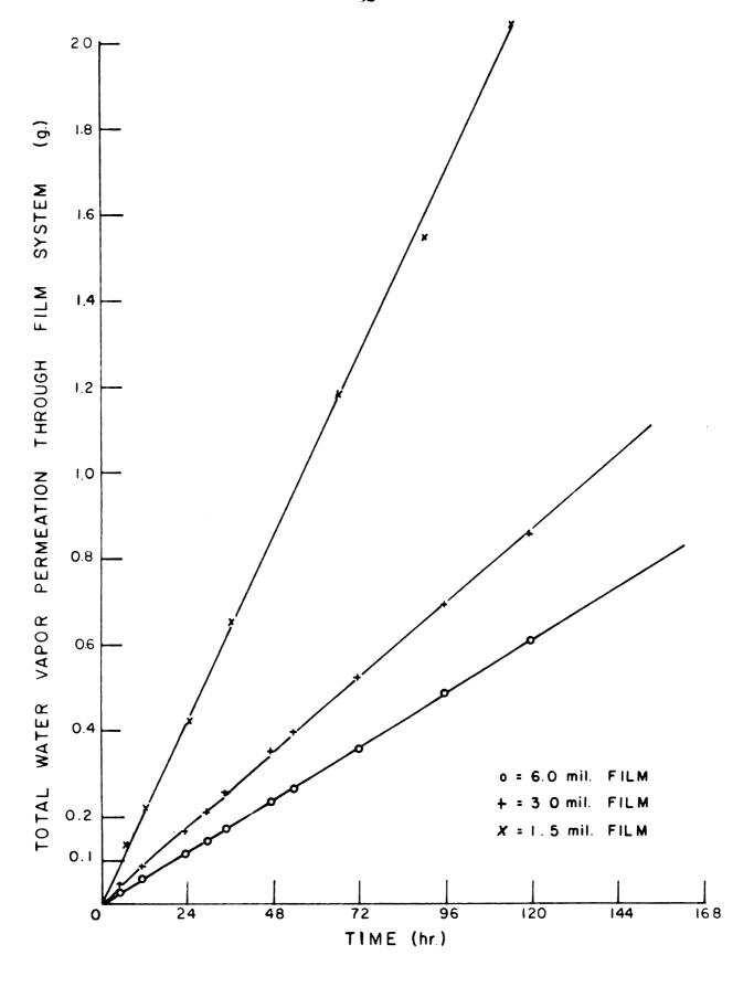
Fig. 8 -- The total water vapor permeation through two different thicknesses of the long oil linseed pur alkyd paint (paint no. 2) on the standard redwood substrate plotted versus the elapsed time.
