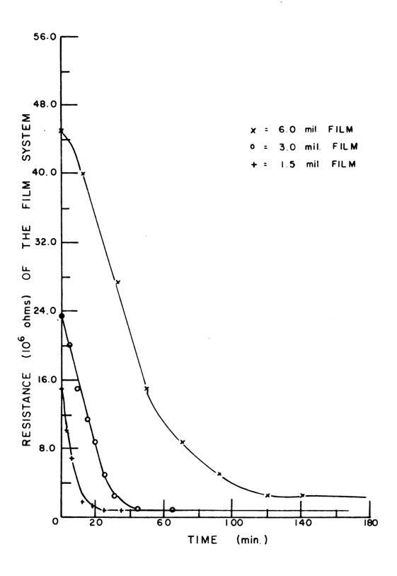
Fig. 18 -- The total liquid water permeation through three different thicknesses of the long oil linseed pure alkyd paint (paint no. 2) indicated by the resistance decrease was plotted versus the elapsed time.
