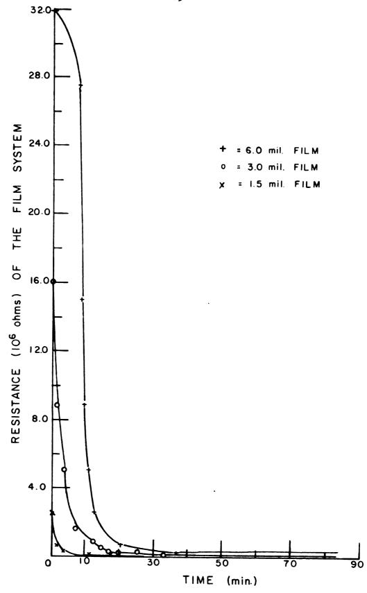
Fig. 19 -- The total liquid water permeation through three different free film thicknesses of the one coat latex (paint no. 3) indicated by the resistance decrease was plotted versus the elapsed time.
