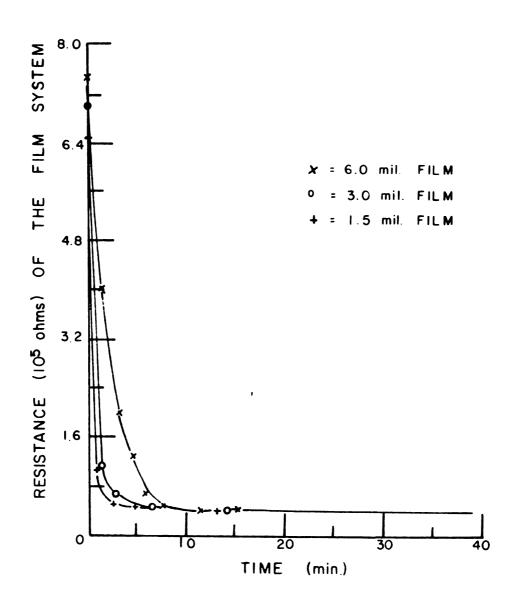
Fig. 20 -- The total liquid water permeation through 3.0 mil. free films of the acrylic emulsion paints (paints nos. 4 and 5) indicated by the resistance decrease was plotted versus the elapsed time.
