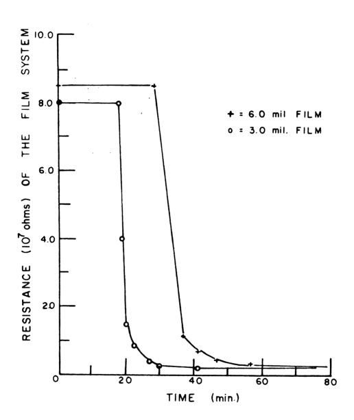
Fig. 22 -- The total liquid water permeation through 3.0 mil. films of the one coat latex paint (paint no. 3) on flat grain, fast and slow growth samples was indicated by the resistance decrease plotted versus time. The permeation through the standard system was plotted for comparison.
