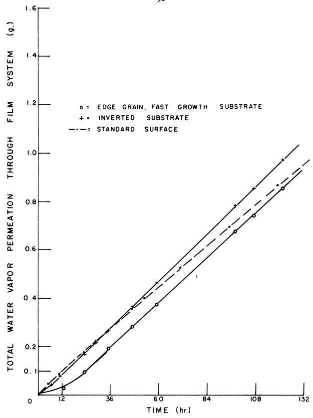
Fig. 15 -- The total permeation through 3.0 mil. films of the linseed oil paint (paint no. 1) on flat grain, slow and fast growth substrates plotted versus the elapsed time. The permeation through the standard system was plotted for comparison.
