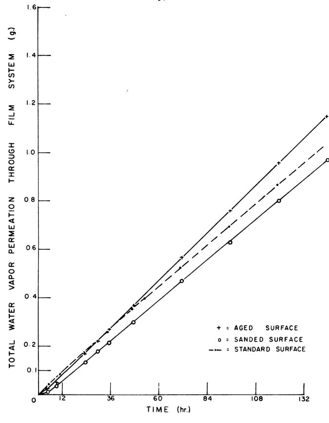
Fig. 12 -- The total water vapor permeation through 3.0 mil. films of the linseed oil paint (paint no. 1) on steamed and sapwood substrates plotted versus the elapsed time. The permeation through the standard systems was plotted for comparison.
