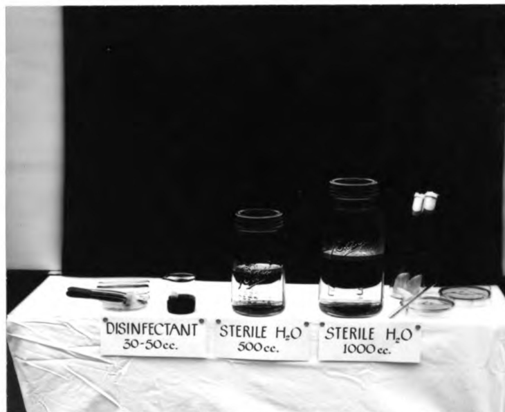
Figure 2. Apparatus used in disinfectant tests with rinse in distilled water.
