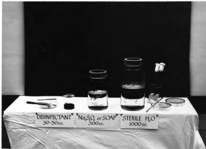
Figure 1. Apparatus for disinfectant tests with rinse in neutralizing agent.
